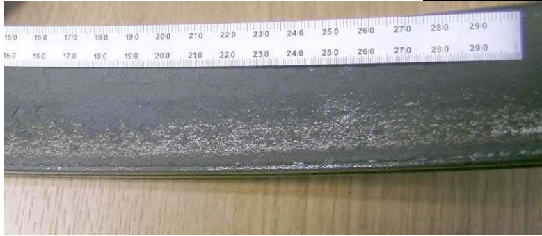
Smearing on the Stage 1 abrasible surface
