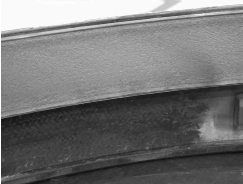
Fig 19 showing remains of the LH Upper Fairing (rear)
