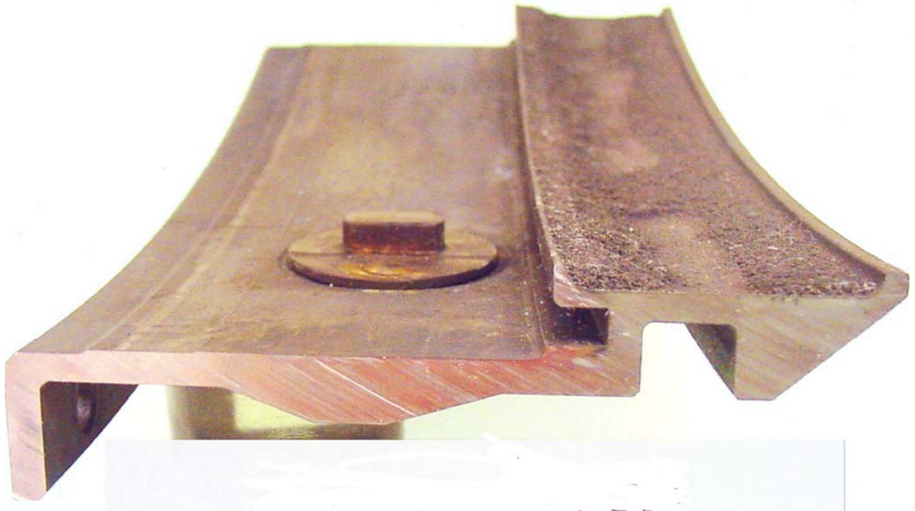
Figure 15 (View 1). Macroscopic views of the #51067 stage 6 compressor ring segment under evaluation at PST. The view shows the cross section of the IN 907 ring substrate, the location of the LCA-314 coated track and the general features of the eroded 314 relative to substrate location. Full ring width is about 3.25 inches, coated track is 1.1 inches.
