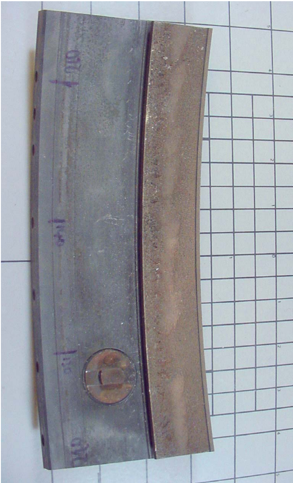
Figure 1. As-received 8.5-inch long segment of stage 6 compressor ring from #51067 Trent 800 engine after flight service with Singapore Airlines. Forward edge on left.
