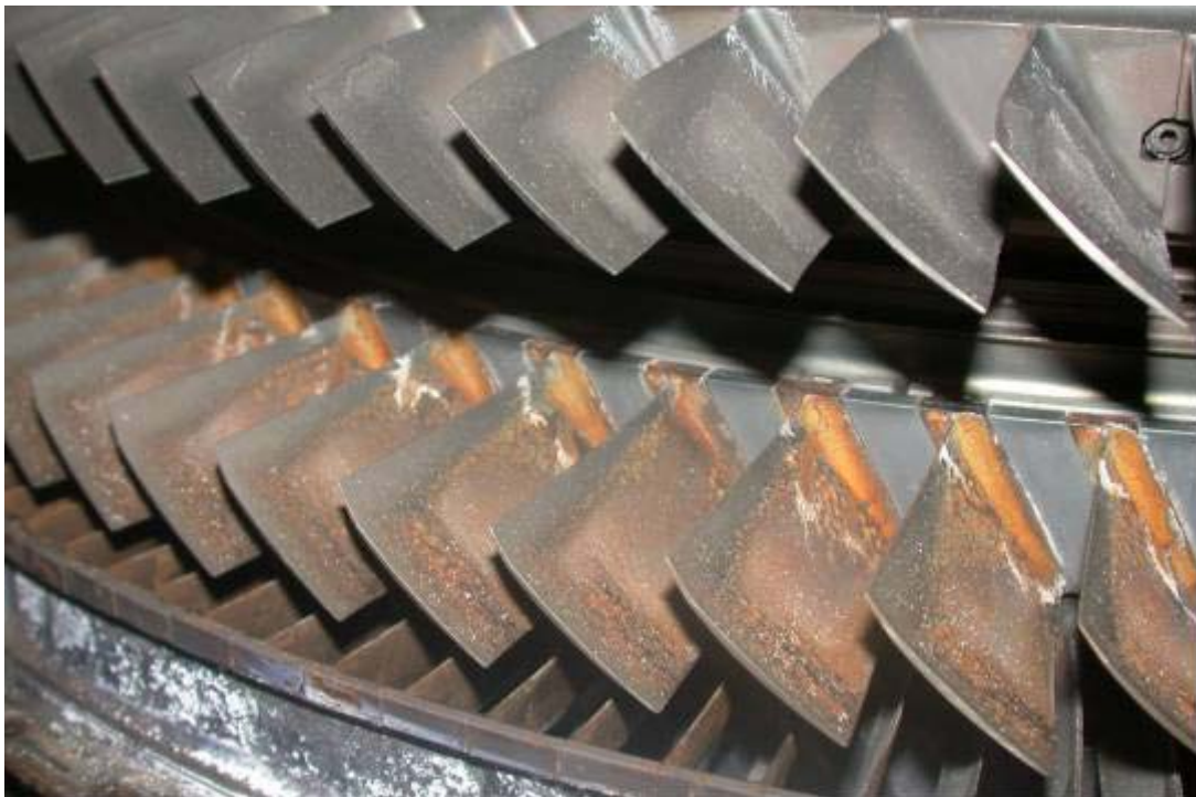
Figure 16 shows an example of a HP compressor stage 3 blade with blueing at the tip
