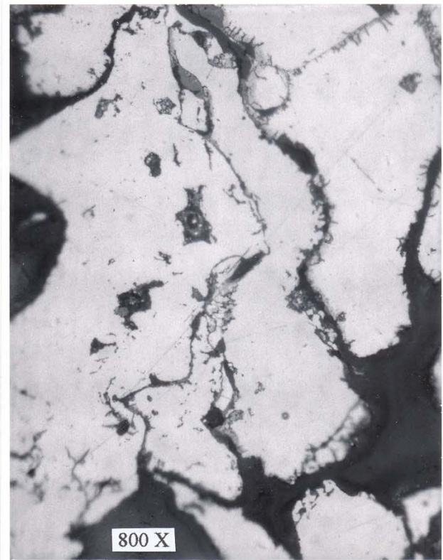
Figure 18b. Optical micrographs of LCA-314 coating chip taken from #51363 stage 6 ring. Detail of NiCrAl phase and severe oxidation formed at splat boundaries during engine operation. Magnification as noted X 0.91.
