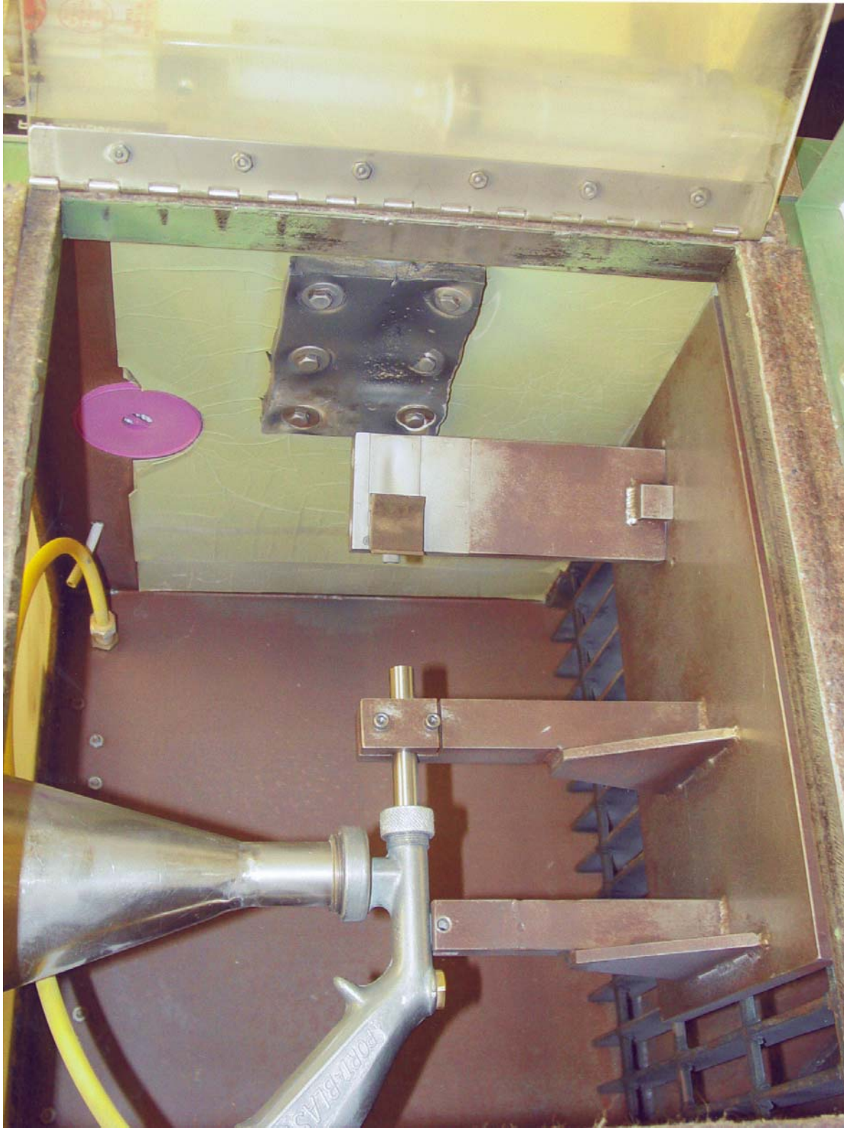
Figure 30. Low angle erosion test rig at PST, with segment of wear track of #51067 stage 6 ring with remnant LCA-314 still adhered after flight exposure. Pure air erosion at 500 ft./sec., 340 cfh flow, 20 degree impingement. In this test, aft edge of coated ring was upstream, erosion spot centered on piece is oval.
