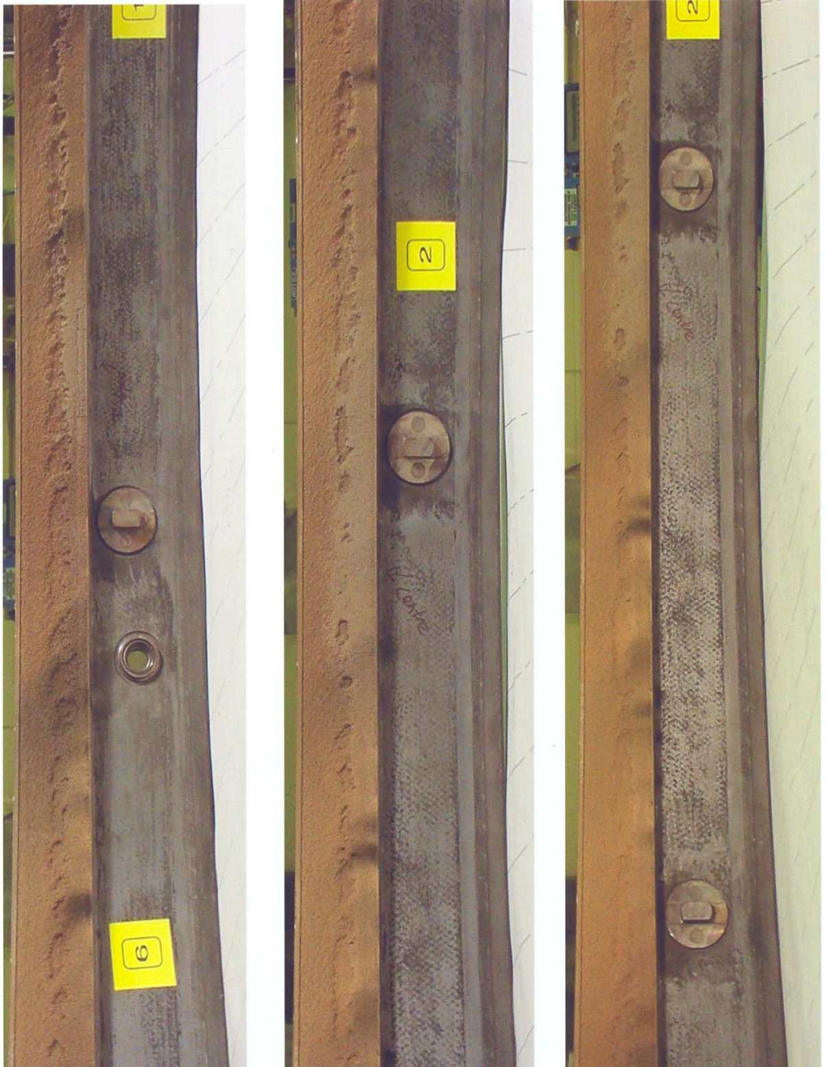
Figure 14. Photographic record of as-received #51363 stage 6 compressor ring with residual LCA-314 coating in upper track area. Whole ring is shown in overlapping views, with PST location numbers. "Pluck-out" of 314 and vivid brown surface coloration are both shown.
