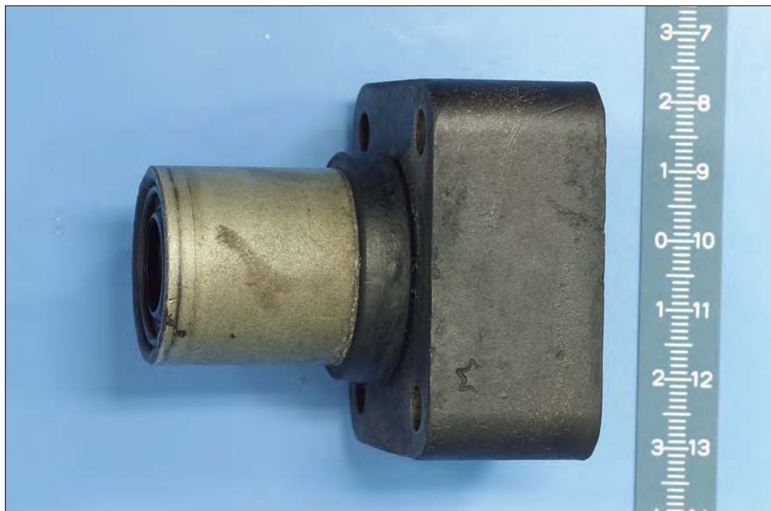
FIGURE 2: Body assembly showing surface discolouration from the post-accident fire
