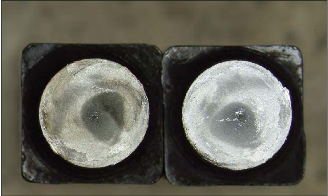
FIGURE 9: Fracture surfaces of the drive coupling
