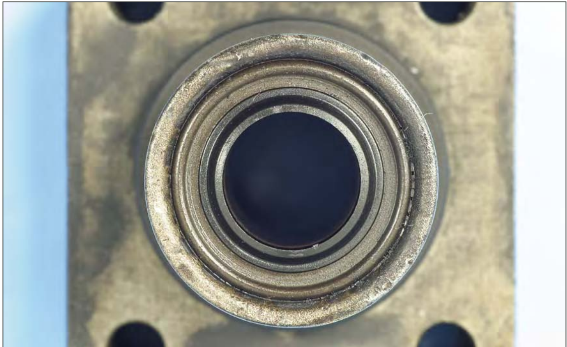
FIGURE 3: Spindle shaft end seal in good condition
