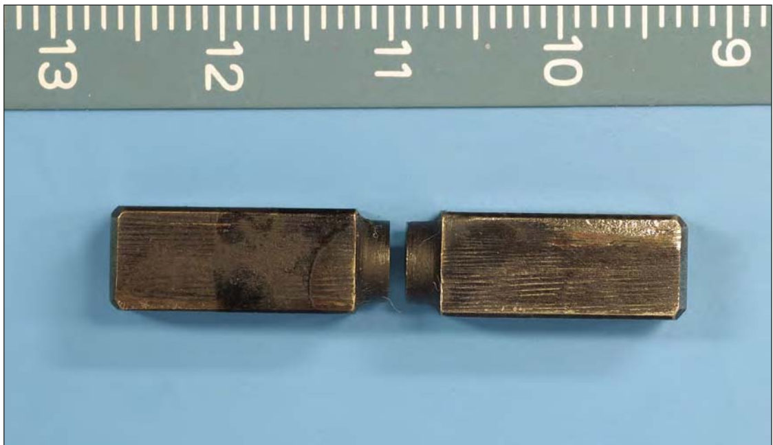
FIGURE 8: Fractured drive pin as recovered from the right EDFP
