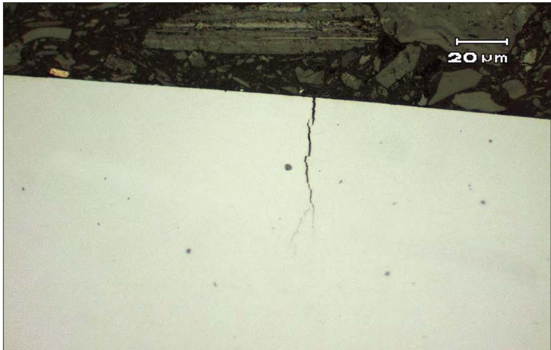
FIGURE 24: Cross section through the area of thermal cracking on the surface of the right EDFP spindle shaft 56
