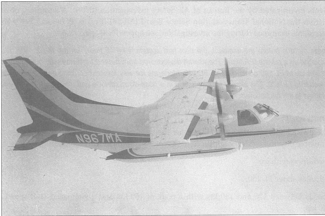
MU-2 aircraft showing commencement of ice accretion on leading surfaces
