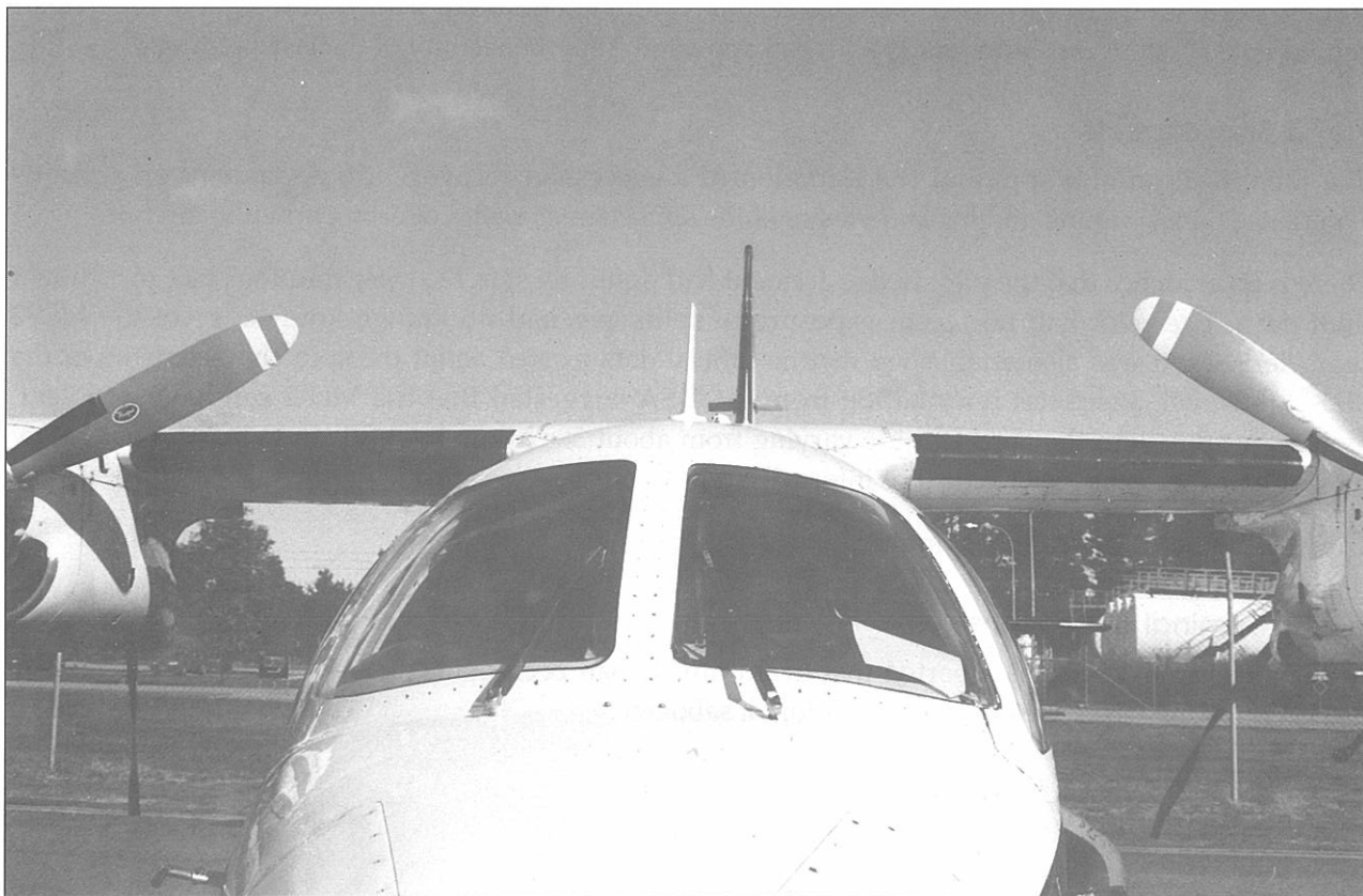
View of de-icing boots on propellers, wings, vertical and horizontal stabilisers.
