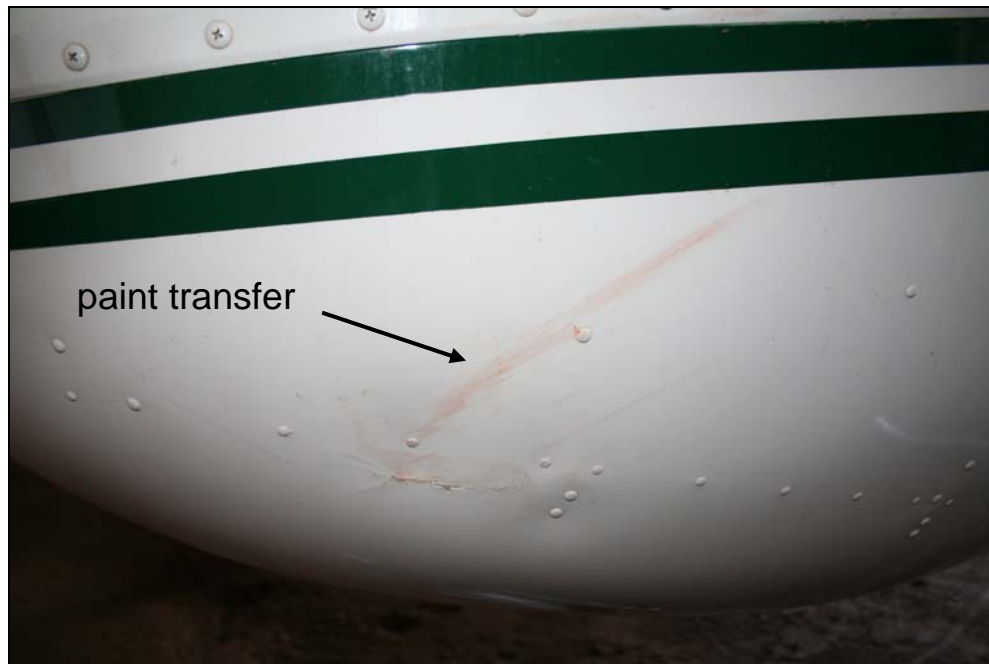
Figure 10: Chin bubble paint transfer
