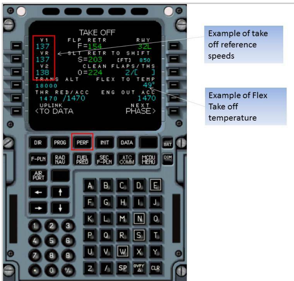
Figure 2: MCDU Performance page: Examples of take-off speeds and flex temperature
