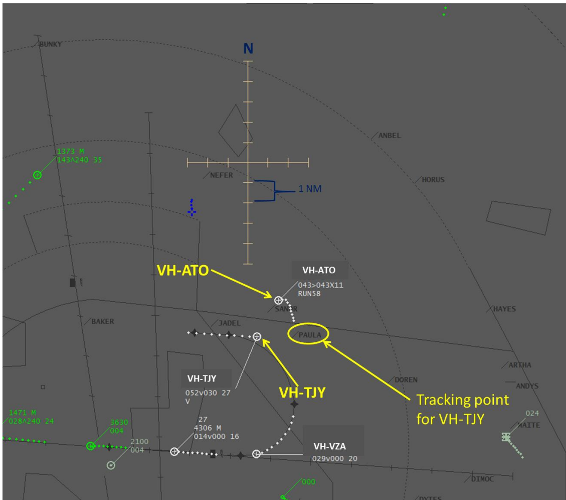
Figure 5: Surveillance display highlighting VH-ATO and VH-TJY and the tracking points for the ARBEY STAR
