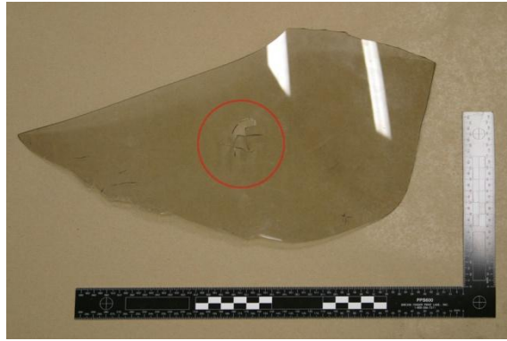
Figure 3: The punctured canopy piece referenced in Figure 2
