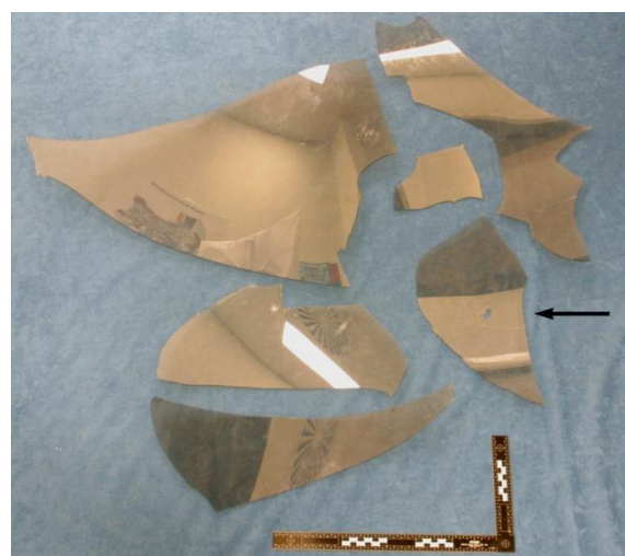
Figure 2: Fragments of the aircraft canopy, as received: note the punctured canopy fragment (arrowed)
