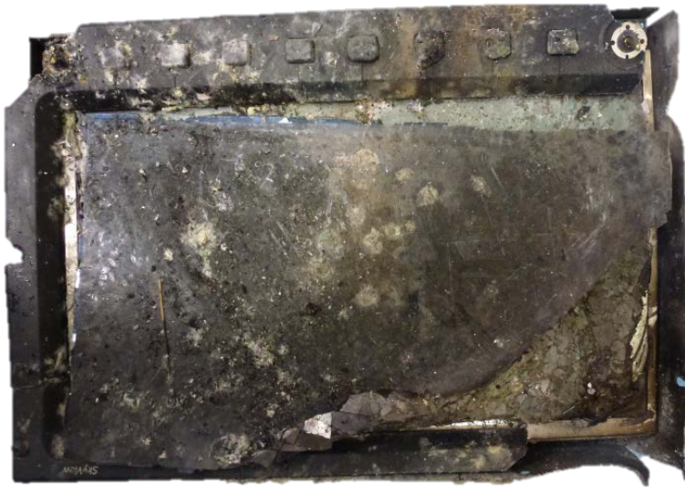
Figure 1: Dynon Avionics display unit – as received
