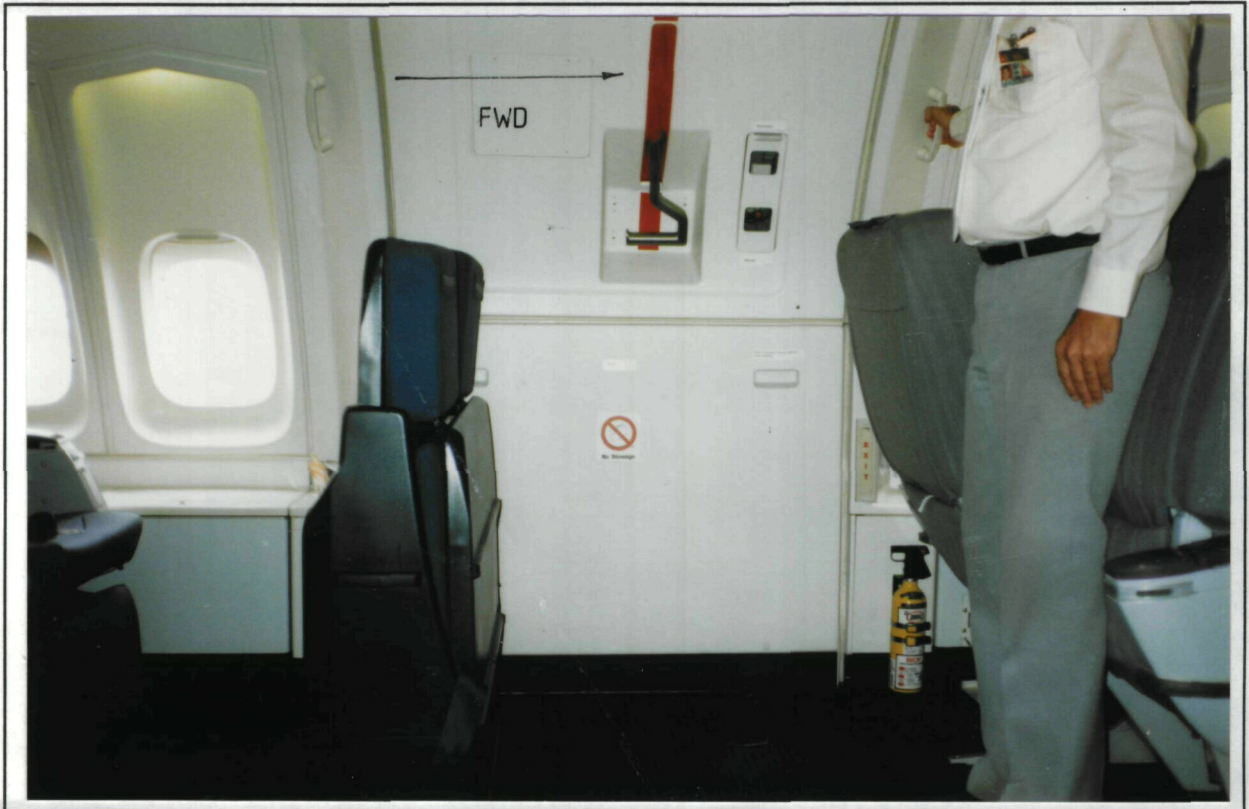
Figure 2. Assist position, new exit seating configuration, upper deck Boeing 747- 400 VH-OJF
