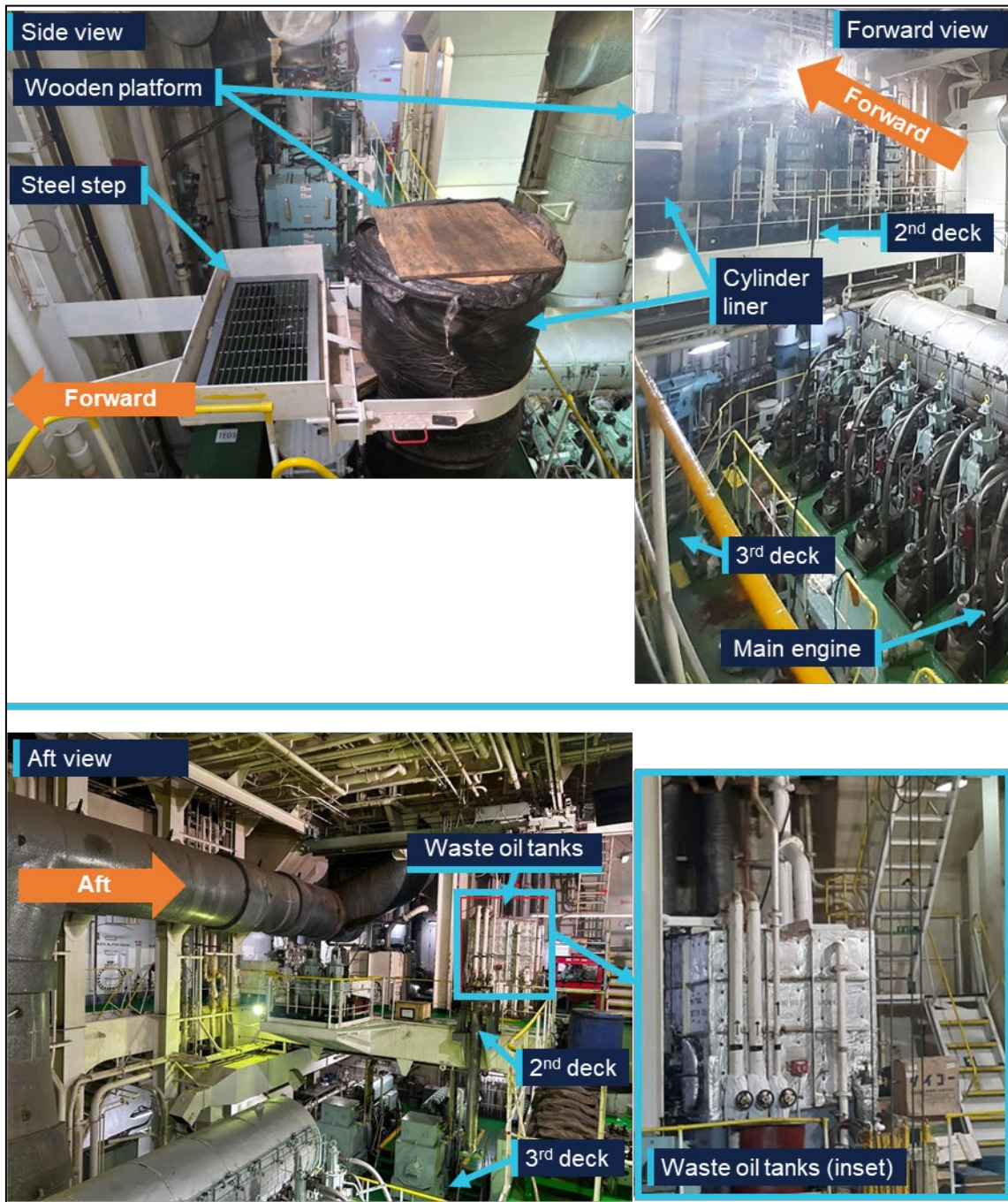
Figure 6: View of engine room – crane access arrangements
