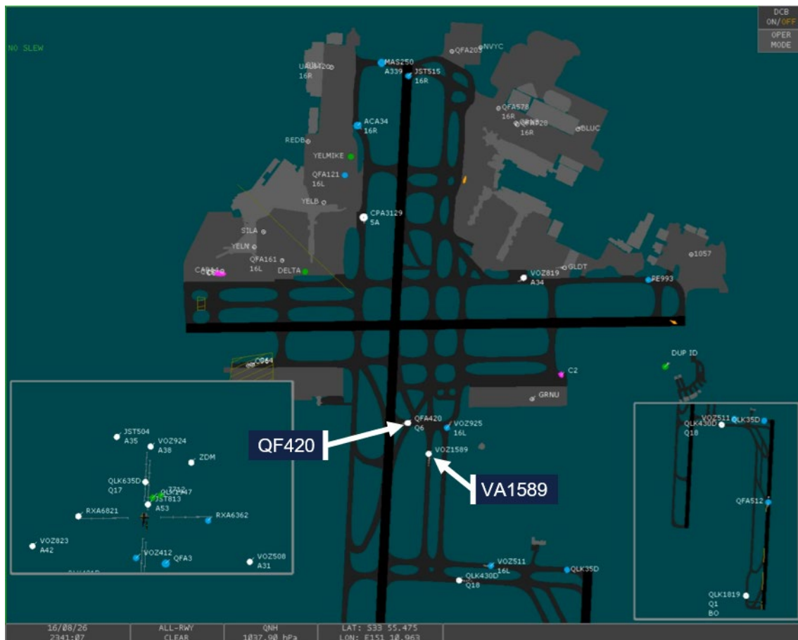
Figure 6: Advanced surface movement guidance and control system prior to the conflict
