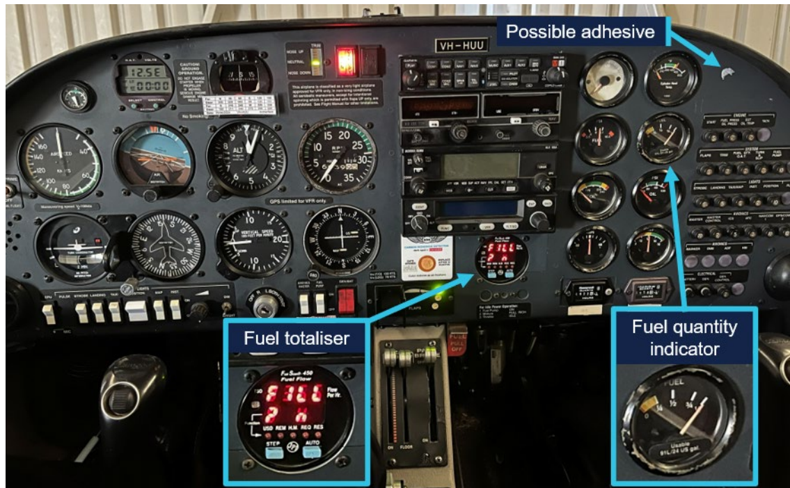
Figure 6: VH-HUU instrument panel
