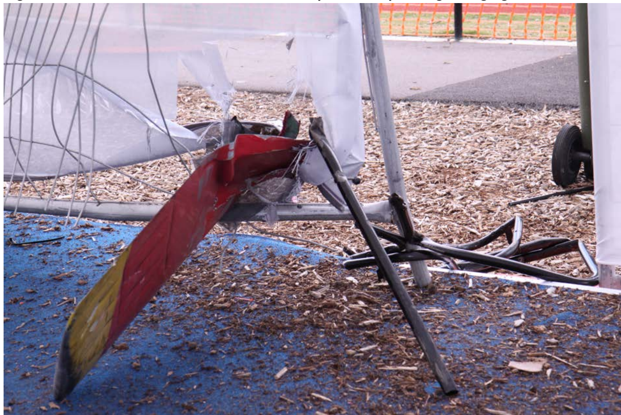
Figure 6: Main rotor debris imbedded in the marquee in the passenger staging area
