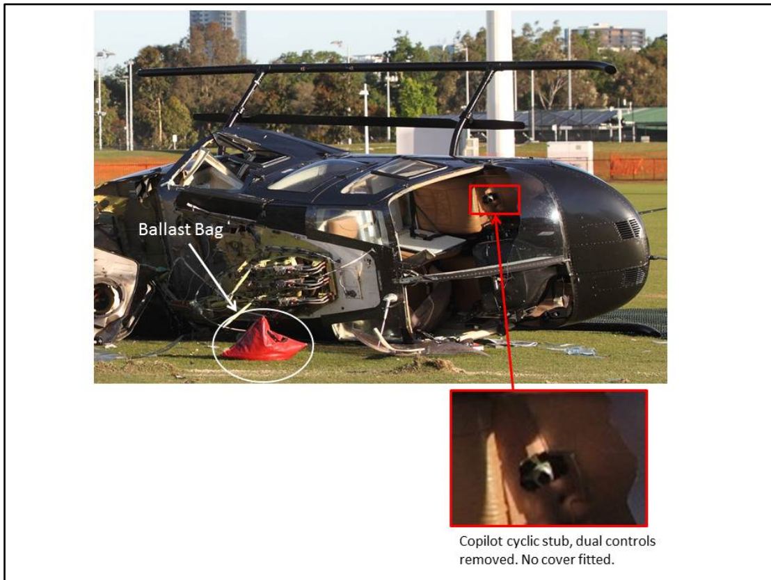
Figure 3: Ballast bag and exposed cyclic control stub (at inset)
