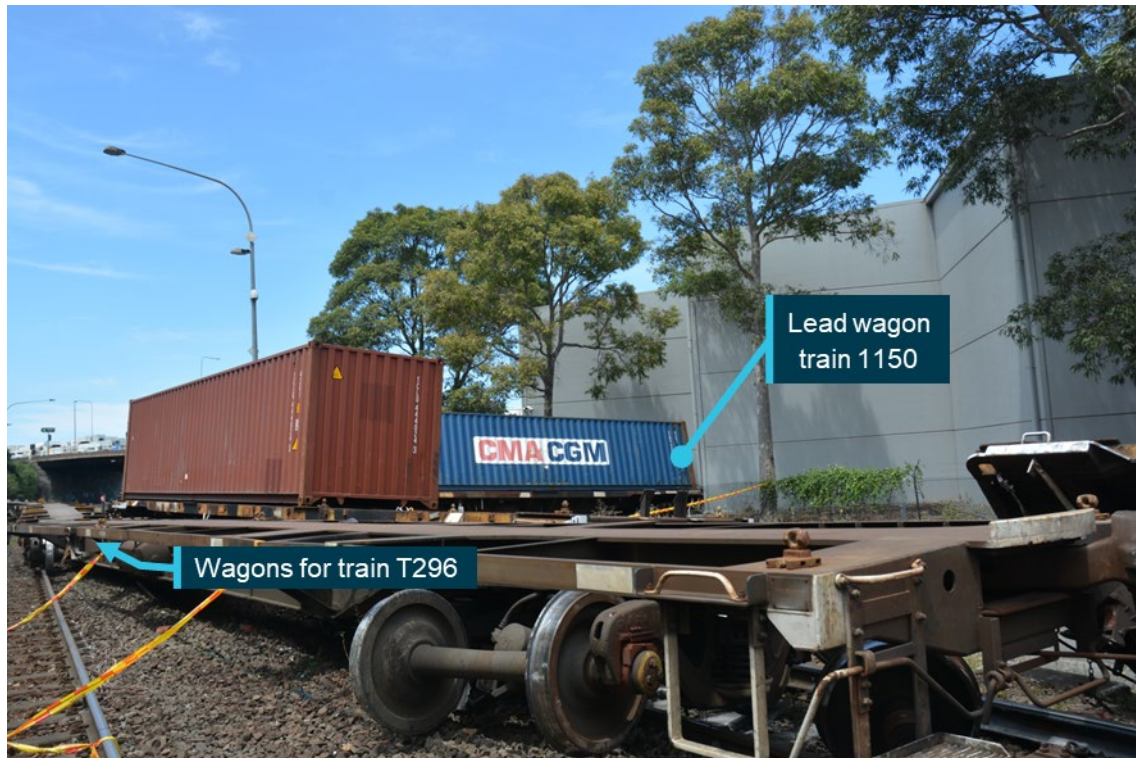
Figure 7: Derailed wagons from trains 1150 and T296
