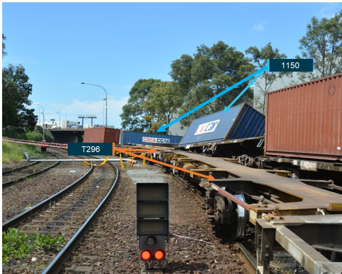
Figure 14: Shunting signal BY29 at stop in Port Botany post-incident
