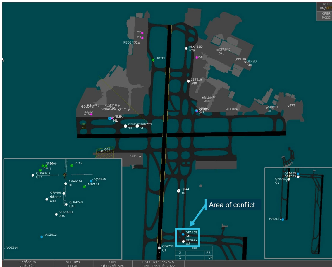
Figure 3: A reconstruction of the A-SMGCS display around the time of the occurrence
