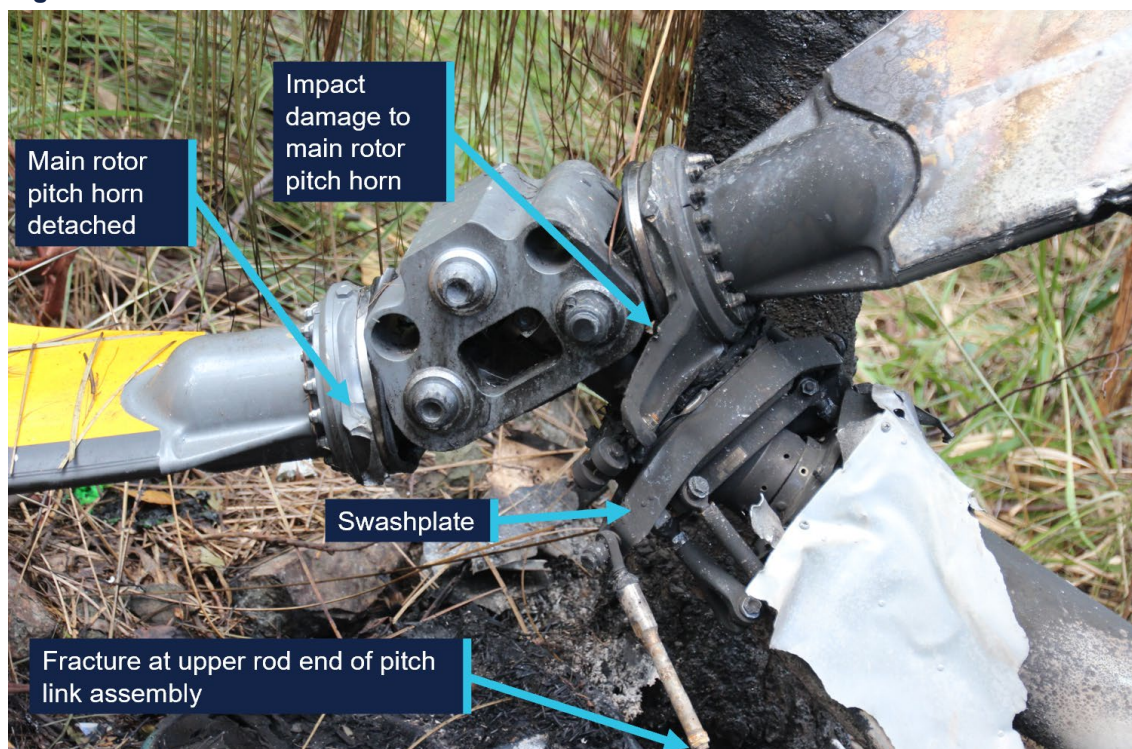
Figure 6: Main rotor hub
