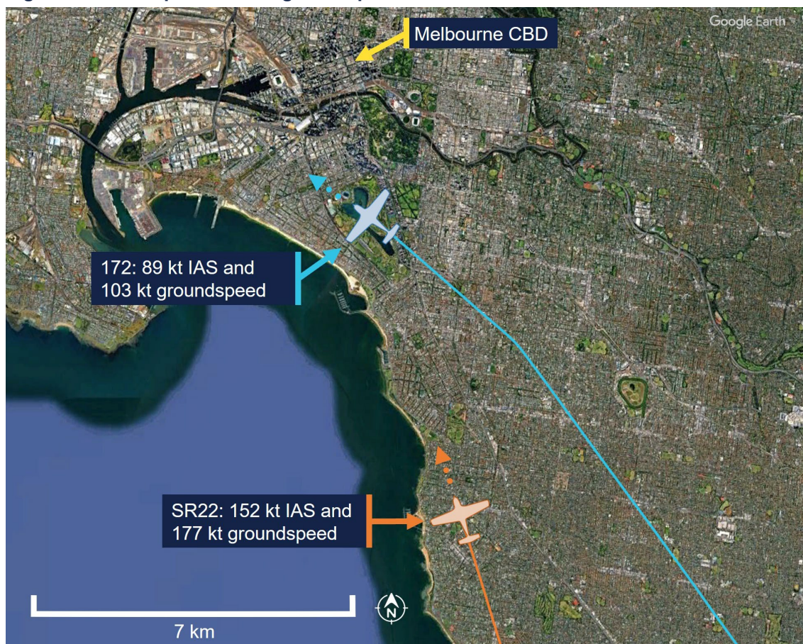
Figure 2: Aircraft position and groundspeed at 2145:02
