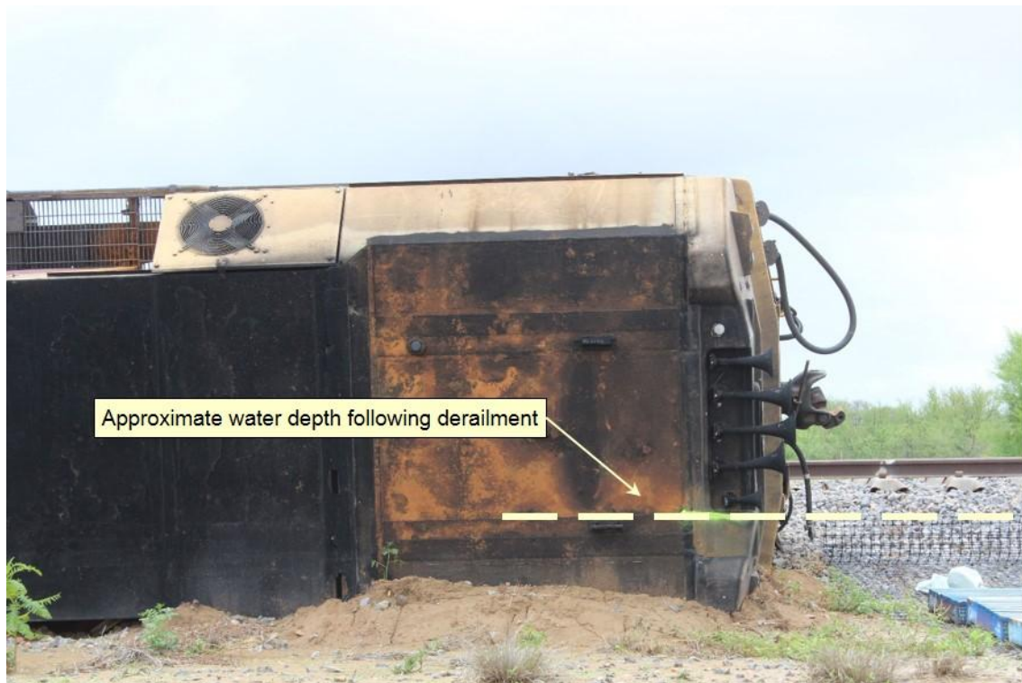
Figure 13: Approximate water depth following derailment
