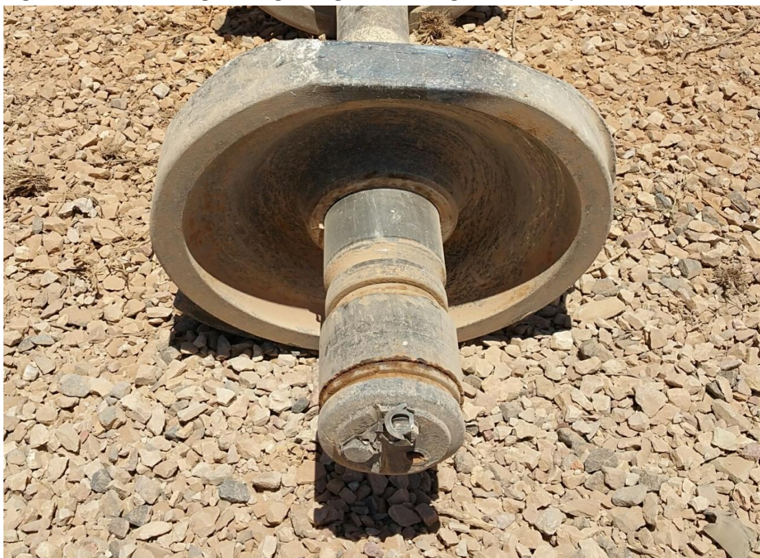
Figure 7: Mated bearing with signs of grease leaking from end caps
