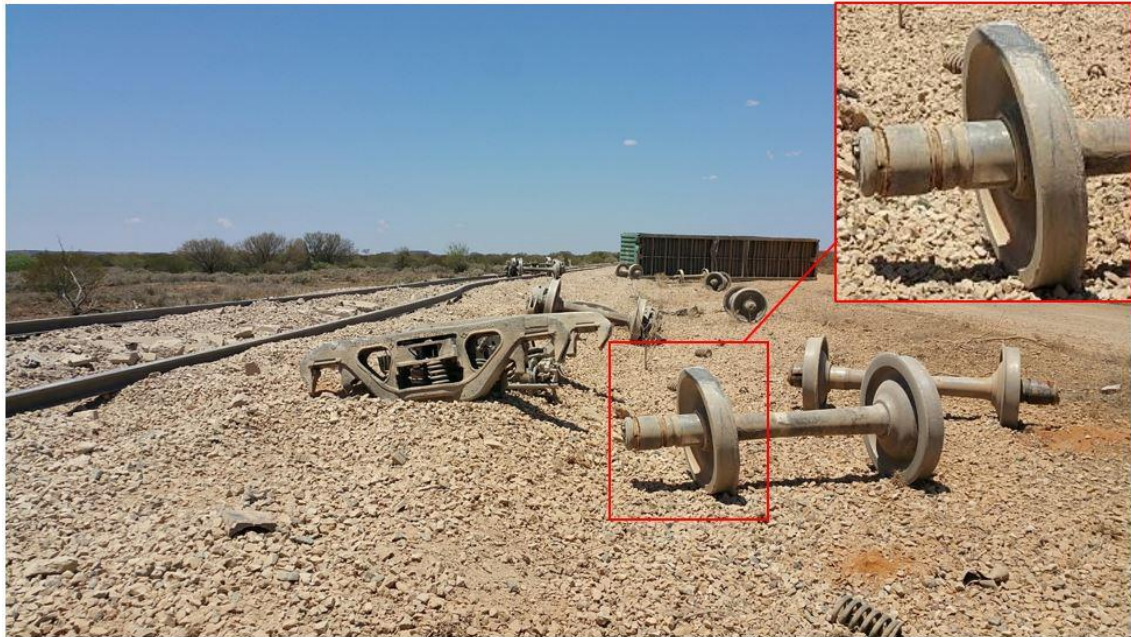
Figure 3: Photo of derailment site with the screwed journal axle in the foreground
