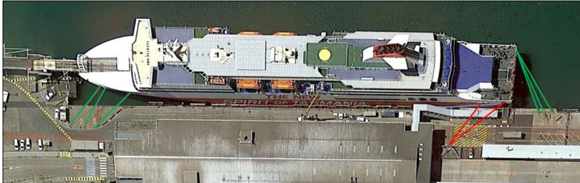
Figure 10: Spirit of Tasmania II 's mooring lines as run on 13 January (lines highlighted)
