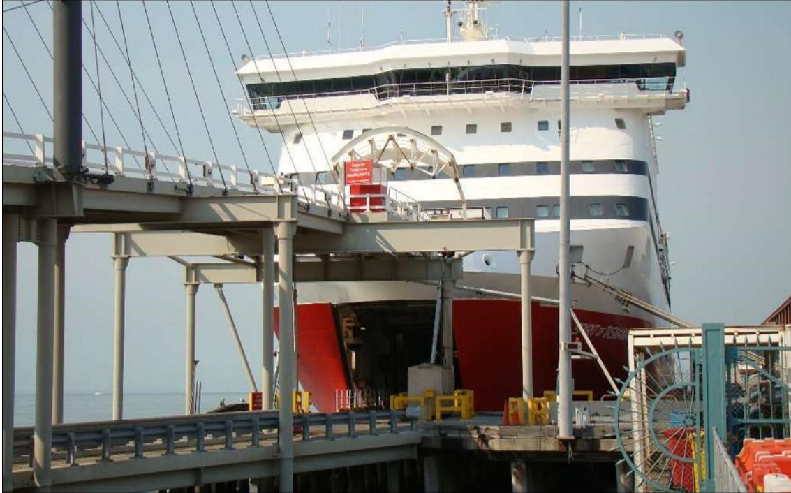
Figure 1: Spirit of Tasmania II 's upper and lower bow ramps deployed at Station Pier
