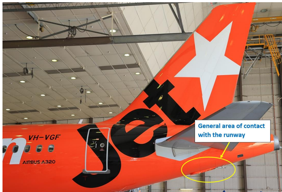
Figure 2: General location of damage
