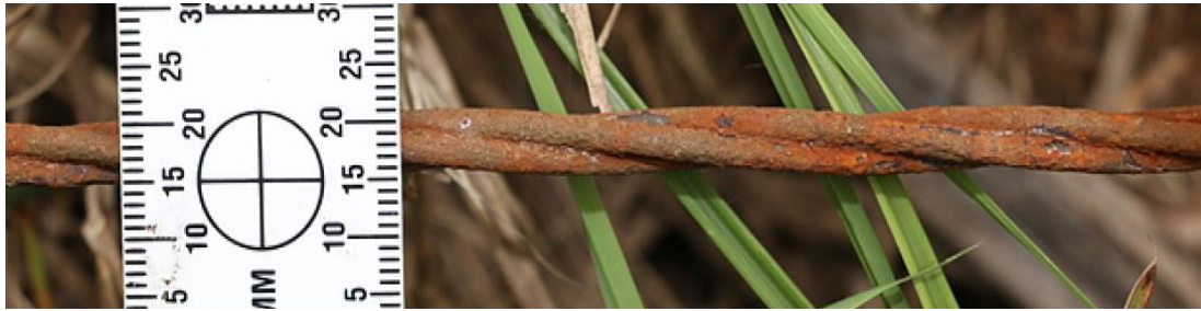
Figure 2: Power cable consisting of three steel wires twisted together (note the rust-like discolouration)
