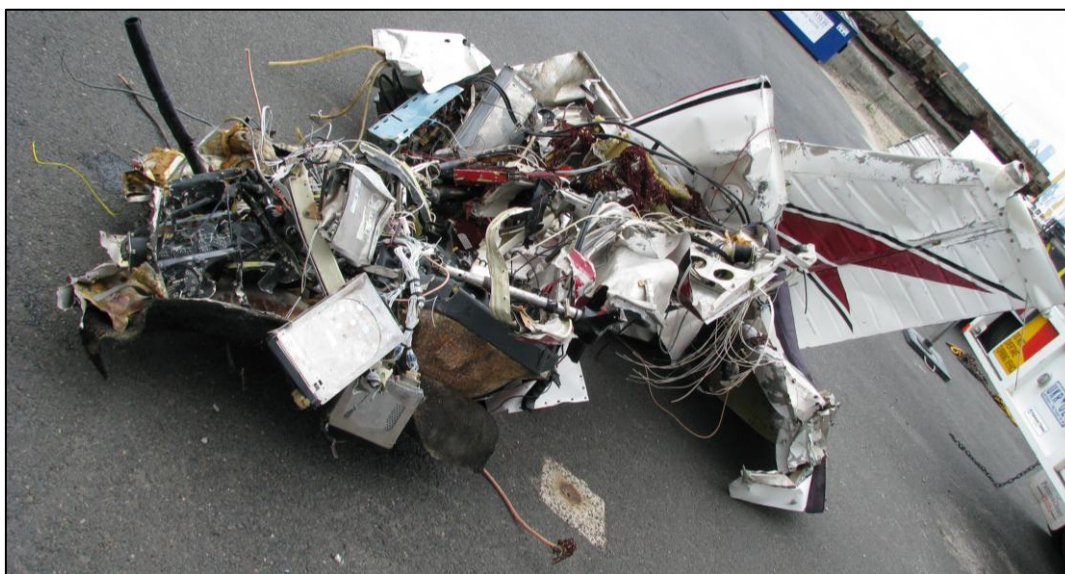
Figure 7: Some of the recovered aircraft wreckage. Note the extent of the disruption of the airframe
