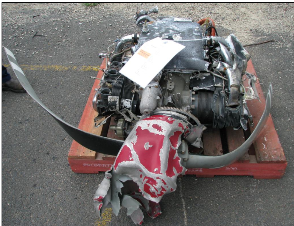
Figure 8: Recovered aircraft engine, propeller and propeller spinner, looking at the lower surface of the engine
