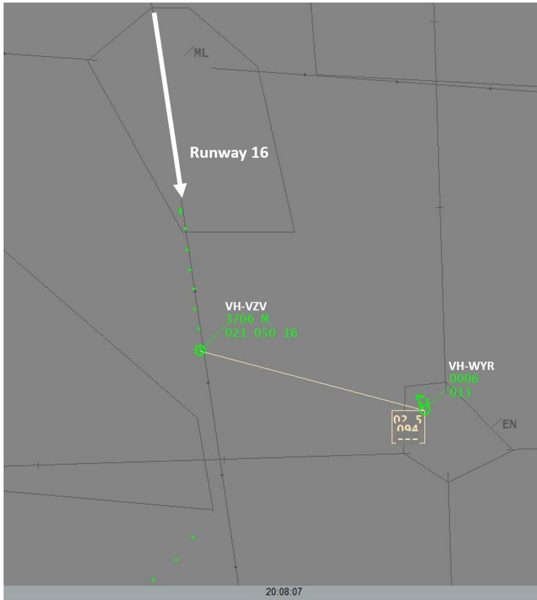
Figure 4: Air traffic control surveillance image at 0708:07, showing VH-VZV 2.5 NM (4.6 km) from and 800 ft above VH-WYR at Essendon Airport 13
