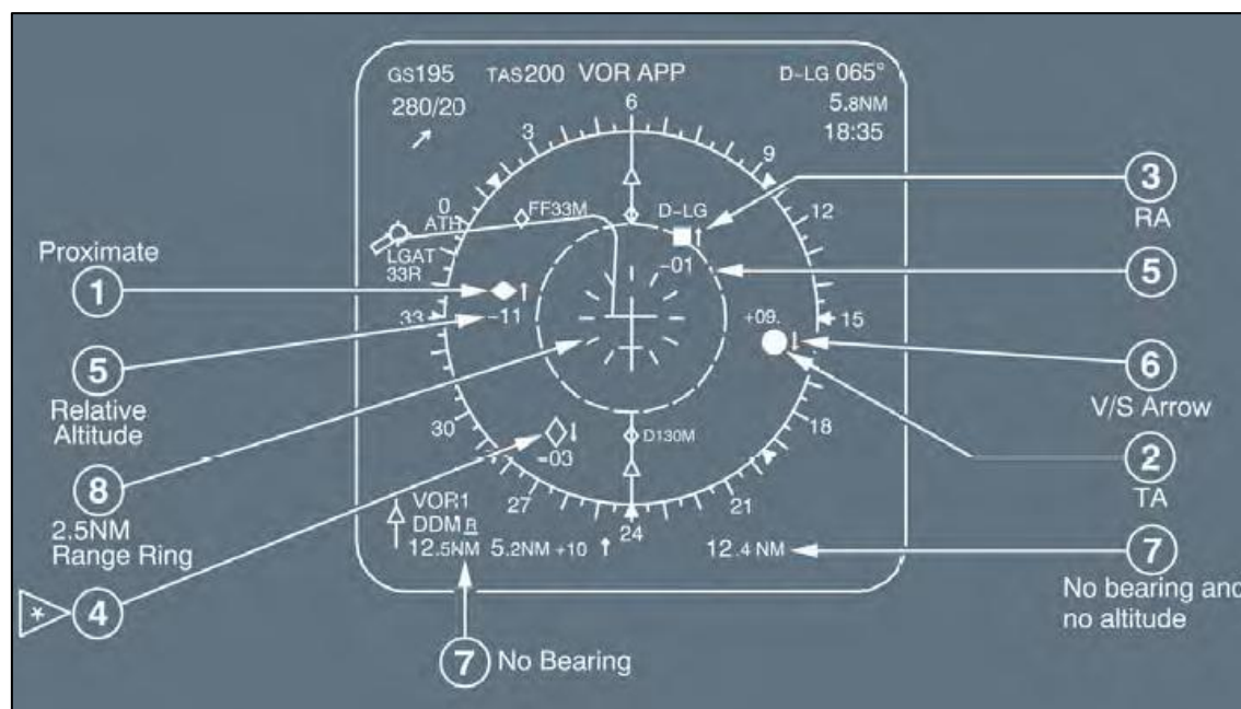
Figure 4: Typical Airbus A320 navigation display depicting the various representations of TCAS intruders. The number of each representation accords with the numbered list above
