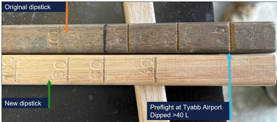
Figure 3: Old dipstick and new dipstick
