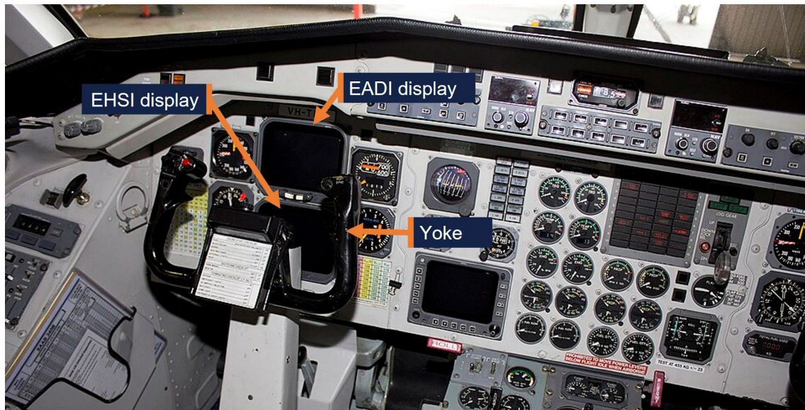
Figure 2: Position of the flight displays relative to the yoke in the forward position
