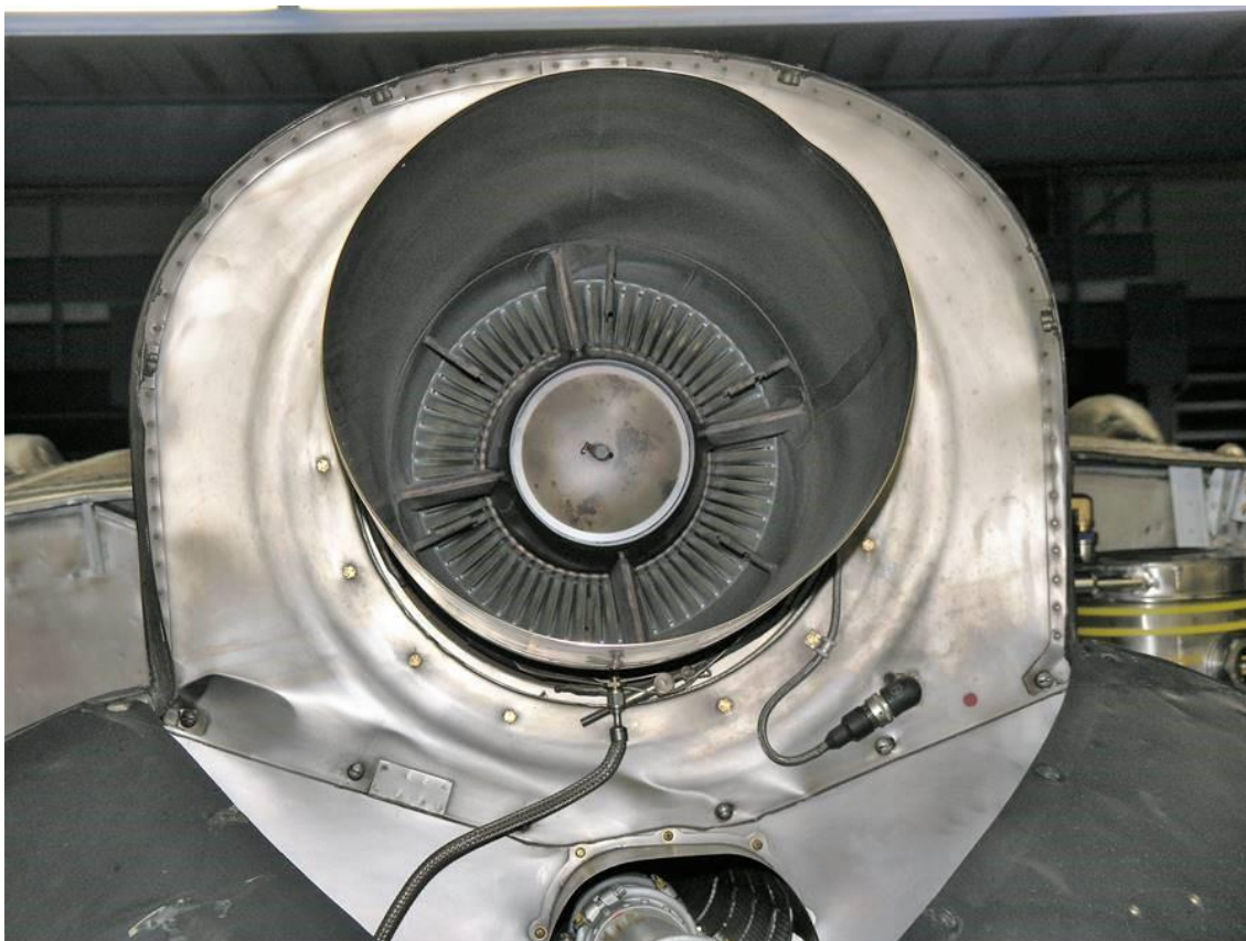
Figure 11: Typical exhaust, showing accessibility for inspection
