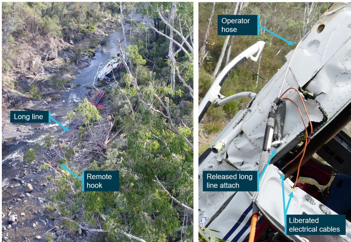
Figure 6: Failed to detach long line
