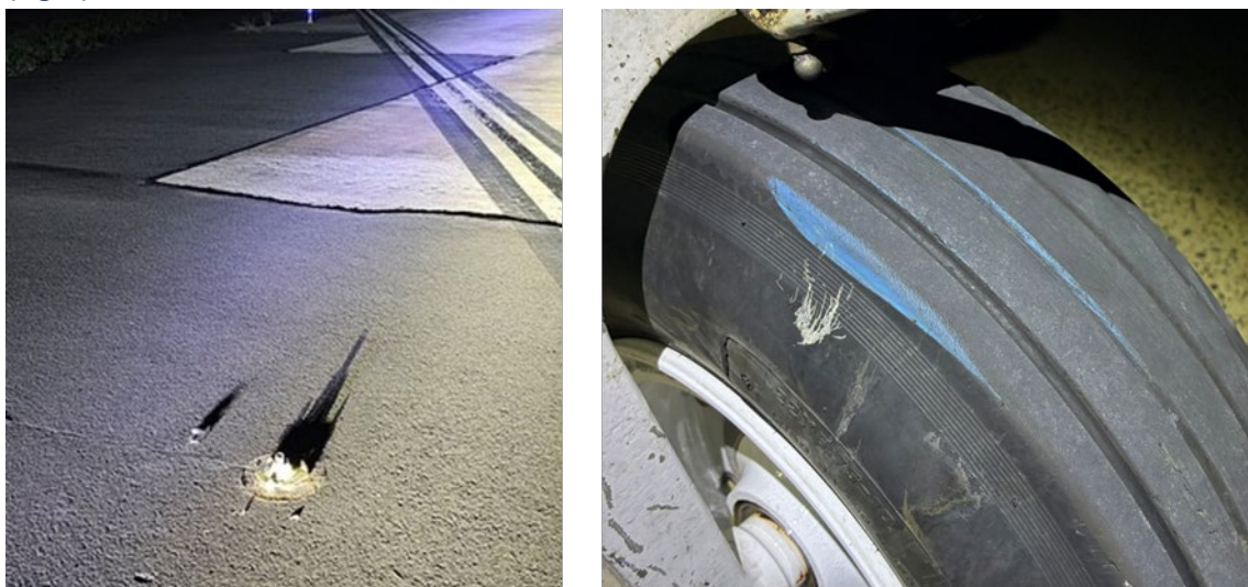
Figure 4: Damaged blue turn node light (left) and blue marks on the aircraft front wheel (right)
