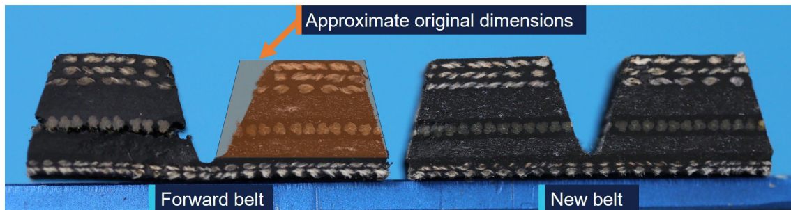
Figure 7: VH-8H8 forward belt cross-section (left) and new rev-Z belt (right)
