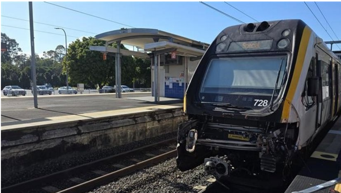
Figure 3: Impact damage to Queensland new generation rollingstock DMB 729
