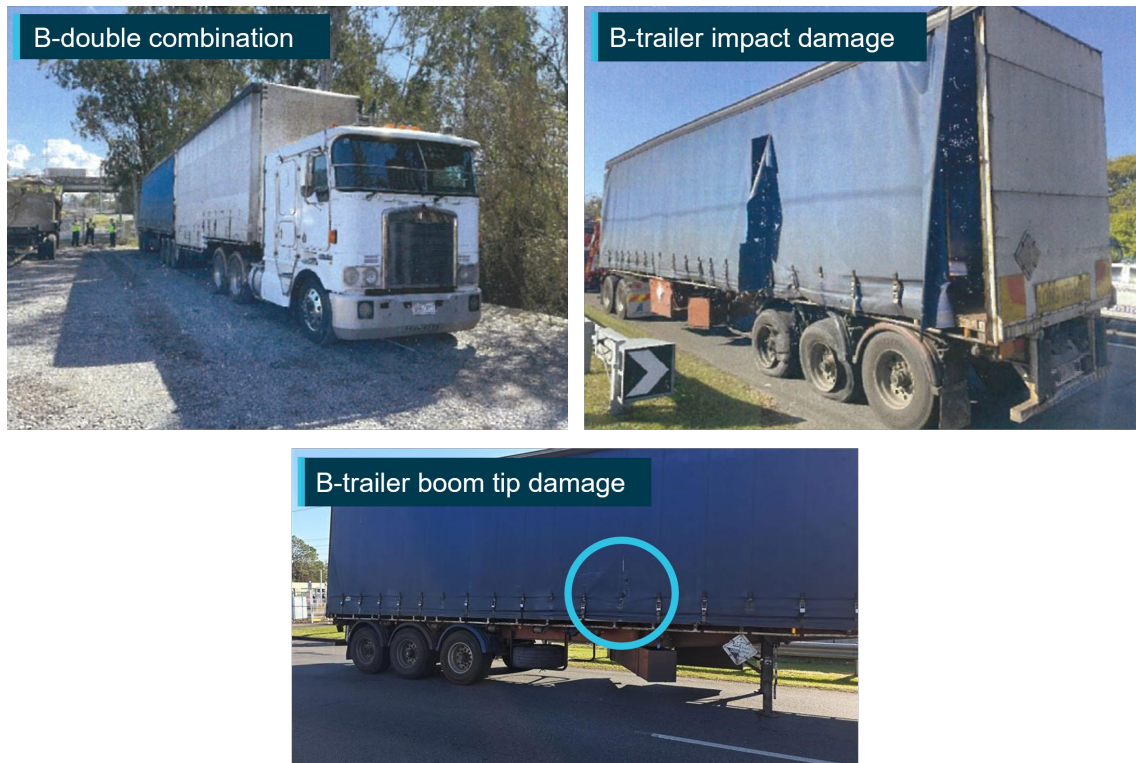
Figure 4: B-double truck configuration and damage
