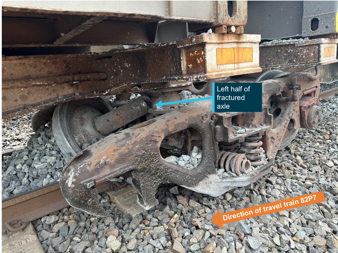
Figure 4: Damaged bogie of RNCY137-T showing half of the fractured axle
