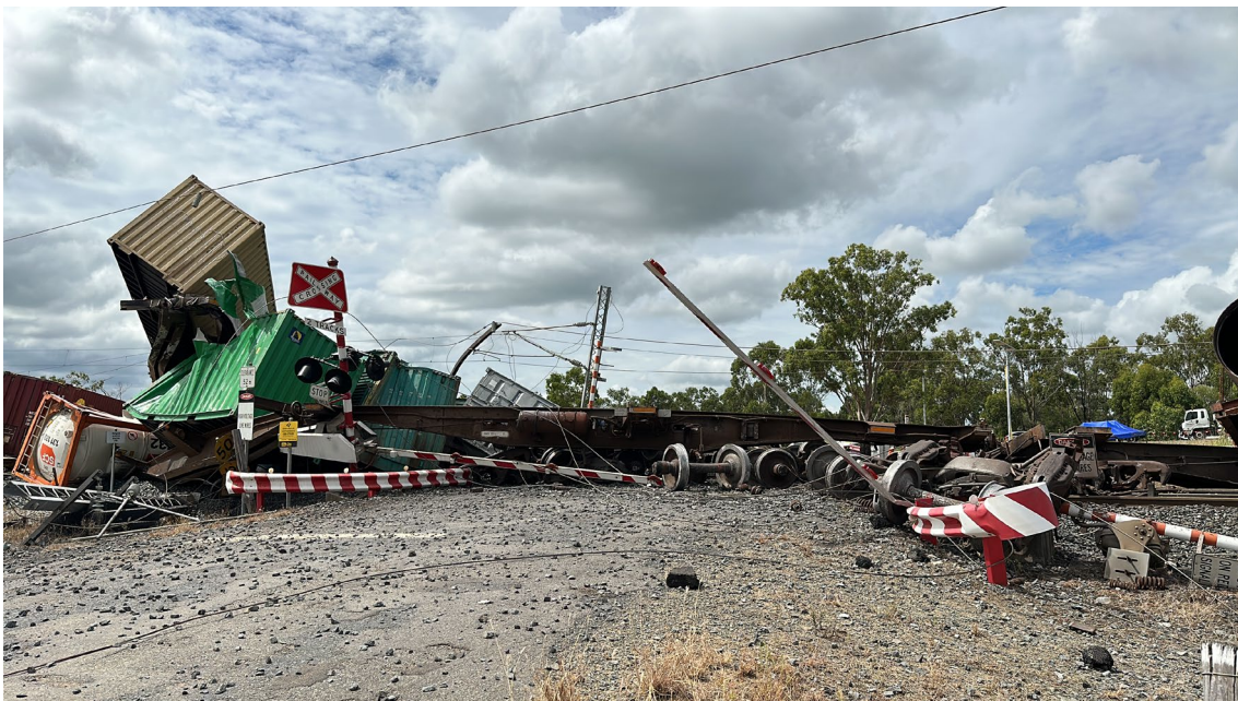
Figure 1: Main wreckage site of train 82P7 at Bills Road level crossing
