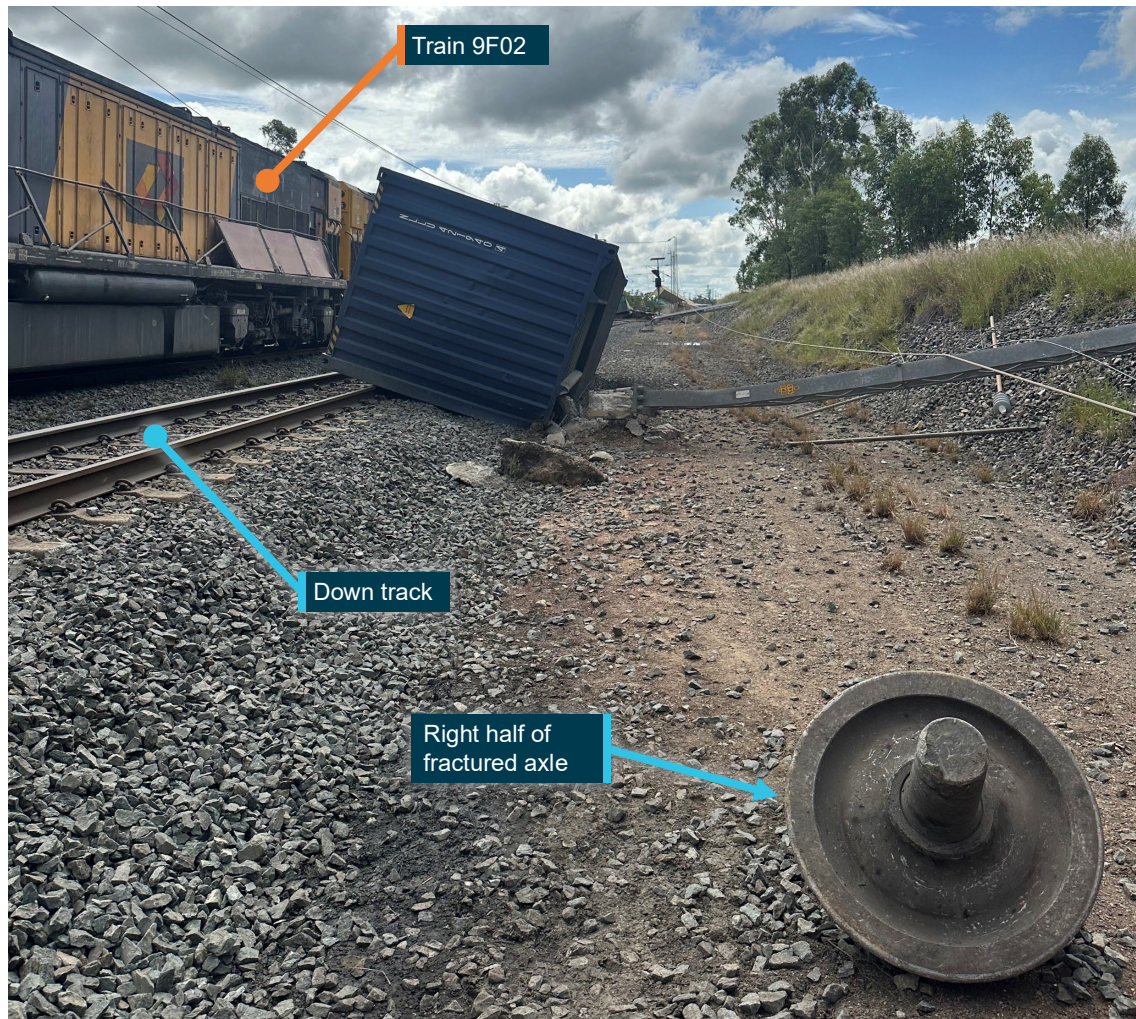
Figure 10: Location of right half of fractured axle from train 82P7
