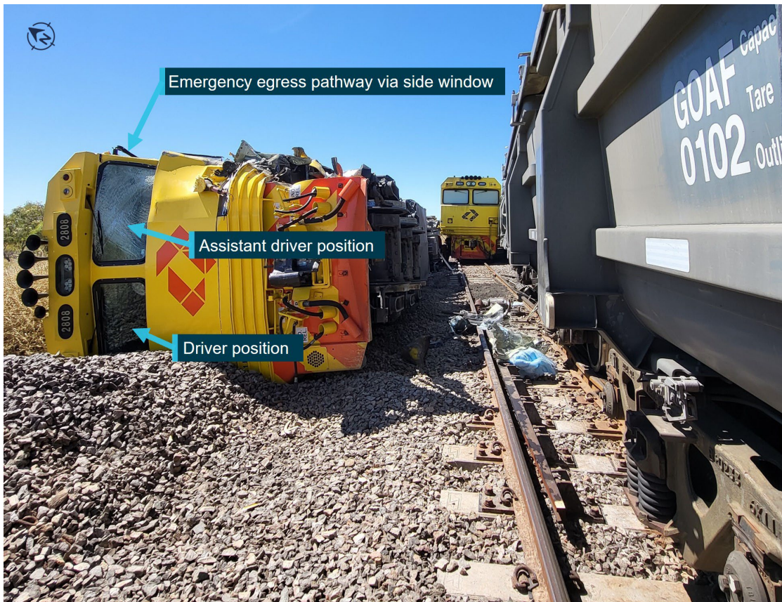
Figure 12: Overturned lead locomotive of train 9M48
