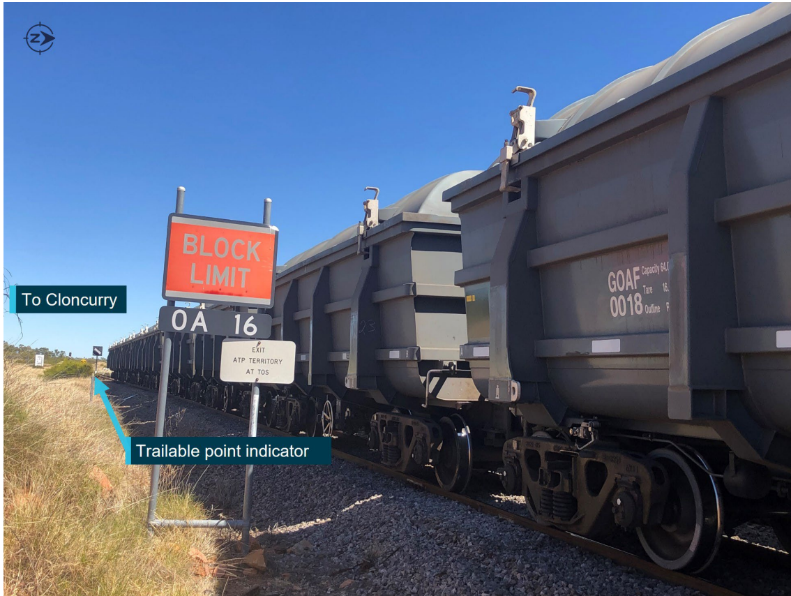
Figure 9: Rear portion of train 9227 showing the wagons were not in-clear of BLB OA 16
