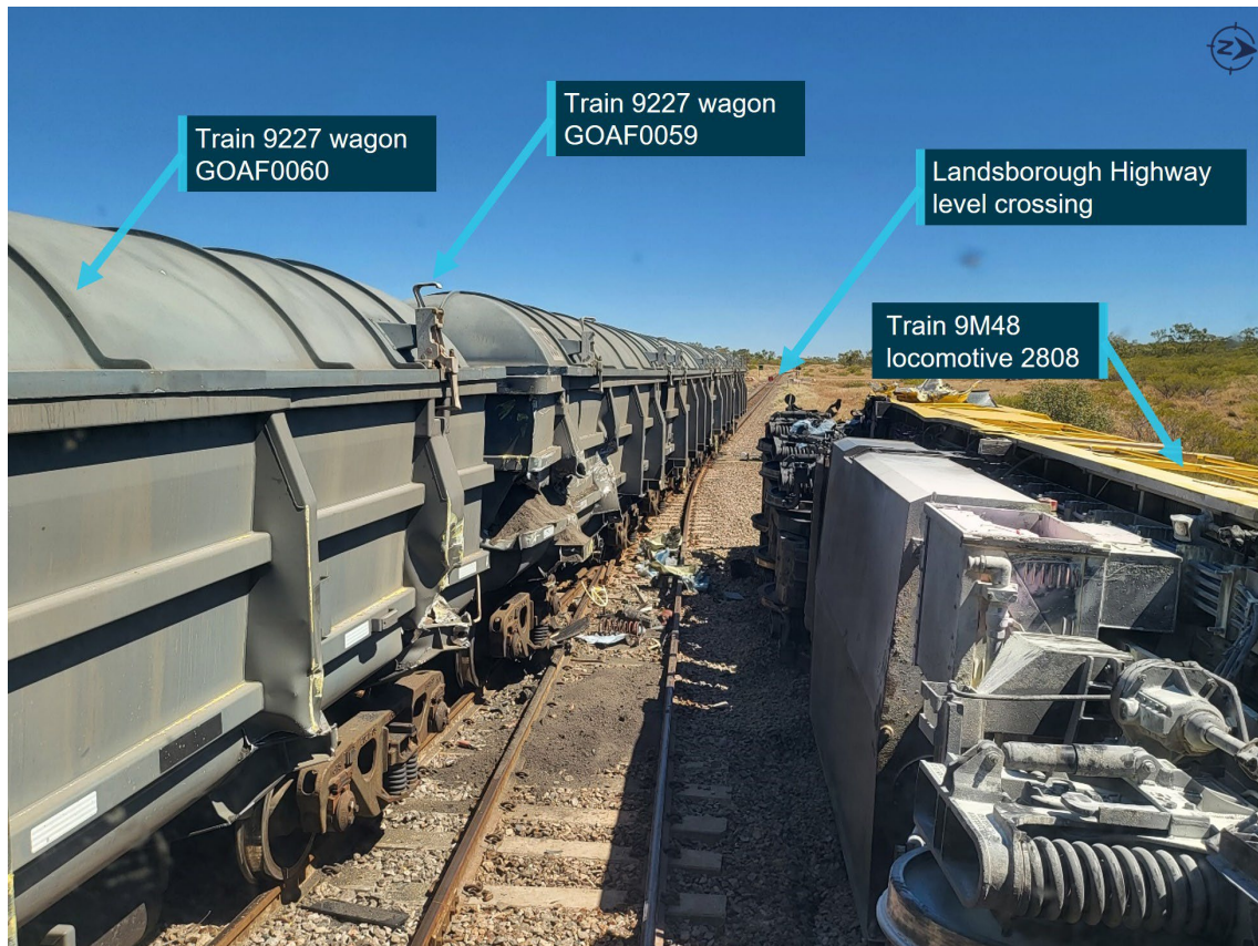
Figure 2: Collision damage to trains 9M48 and 9227
