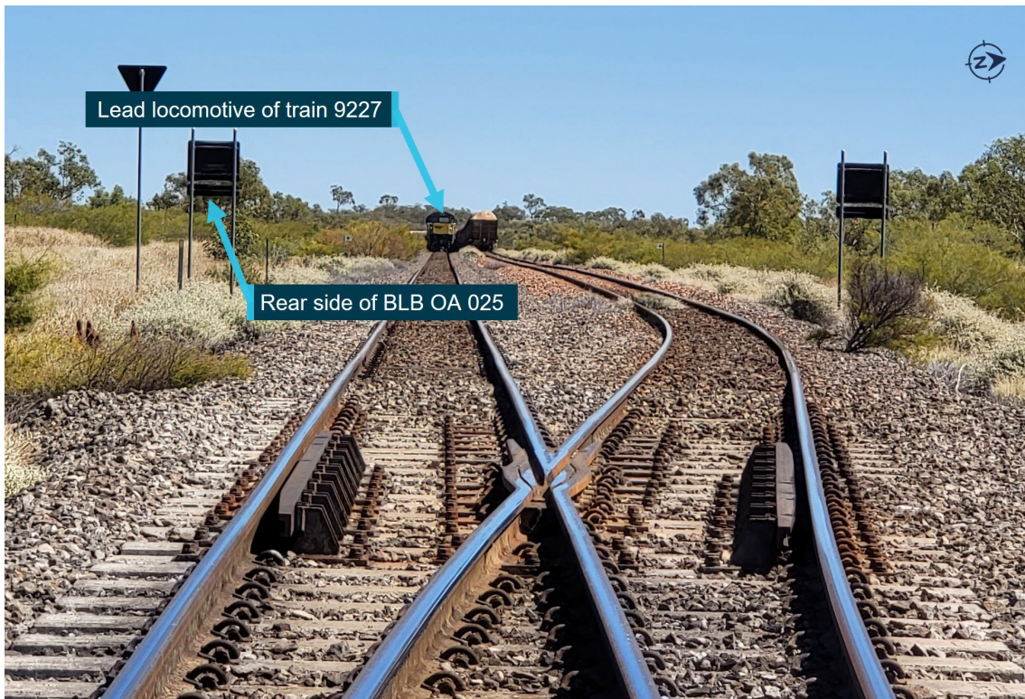
Figure 8: Stopping location of the lead locomotive from train 9227 from the limit of authority at BLB OA 25
