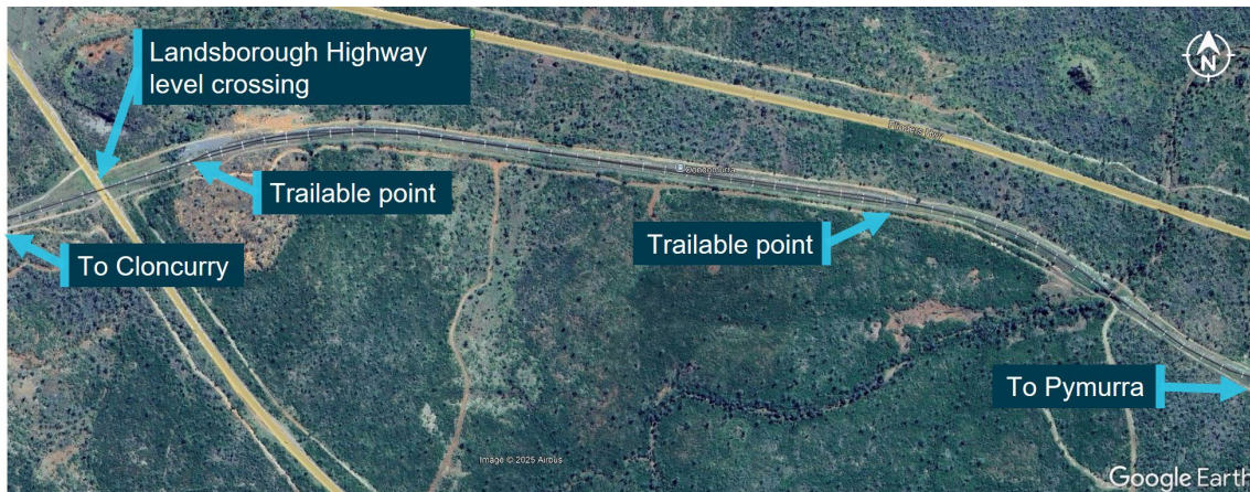
Figure 6: Oonoomurra station track alignment
