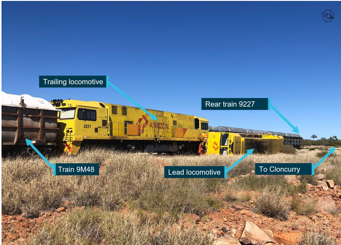
Figure 10: Derailed and overturned lead locomotive 2808 of train 9M48
