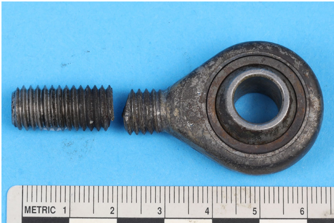
Figure 4: Fractured actuator rod end
