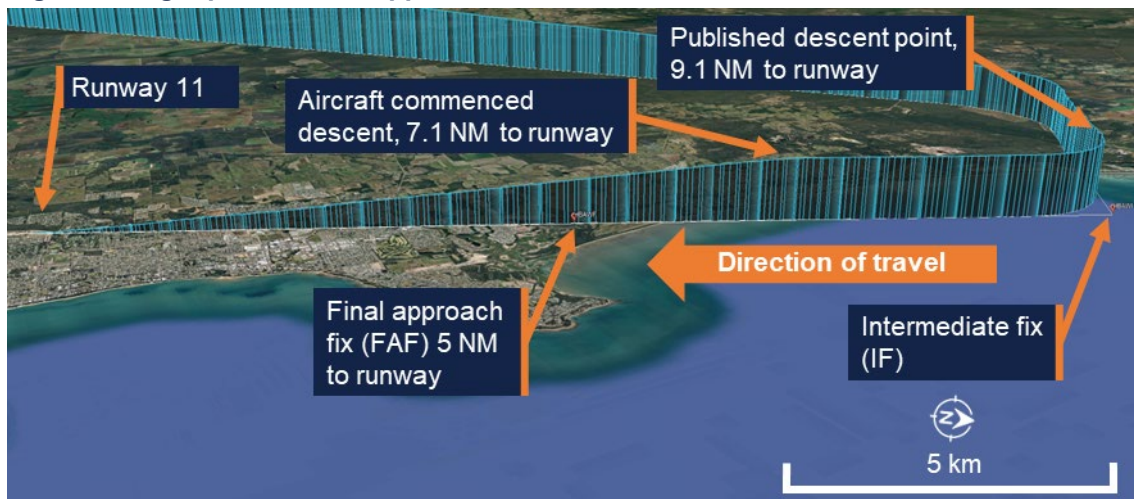
Figure 2: Flight path on final approach
