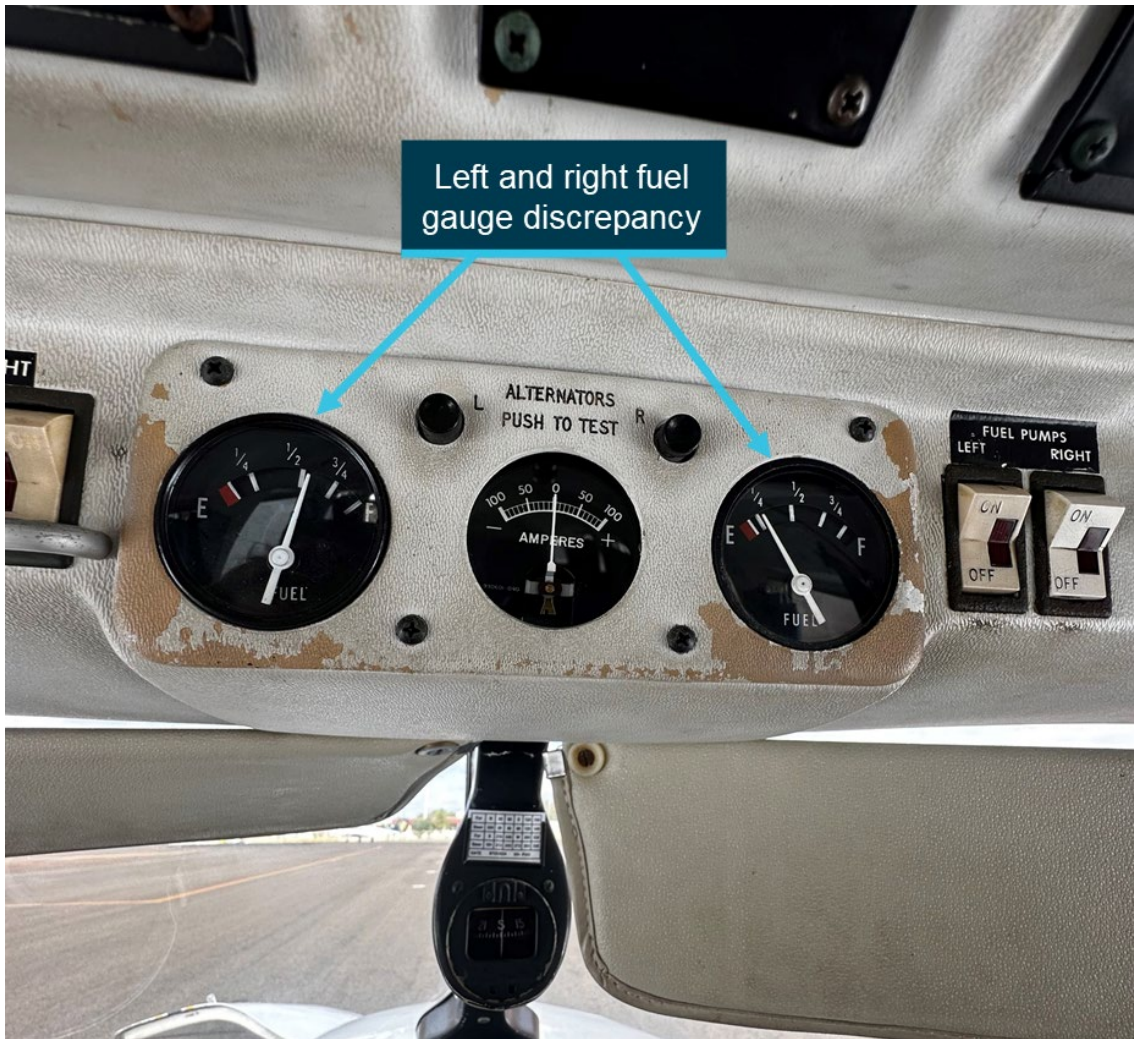
Figure 5: Inboard tank quantity discrepancy after landing
