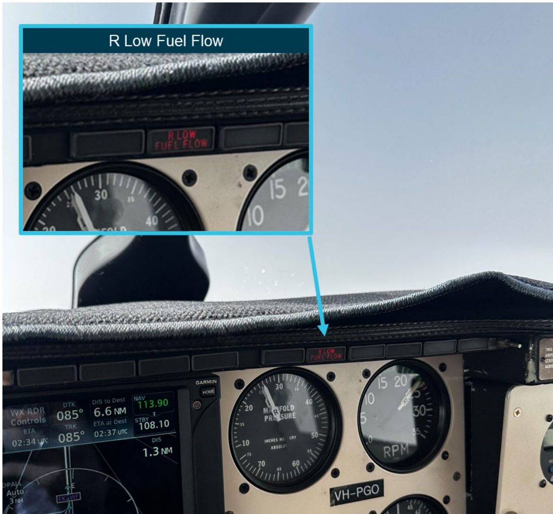
Figure 2: Right low fuel flow annunciator illumination during approach to Meekatharra
