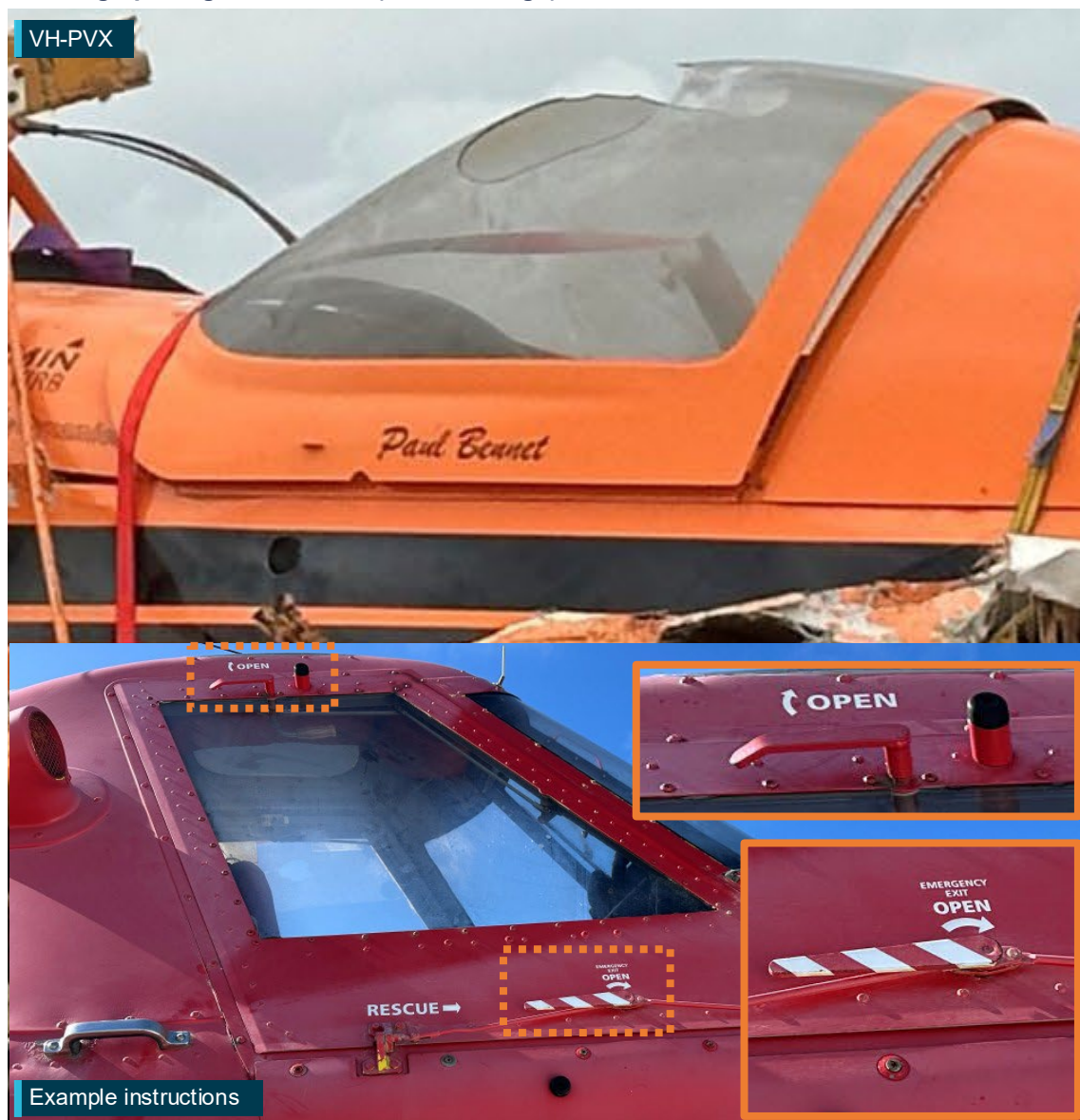
Figure 4: Outside of canopy on VH-PVX (top image) compared with a different aircraft showing opening instructions (bottom image)
