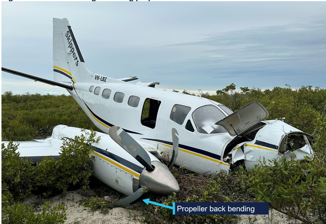
Figure 4: Aircraft wreckage showing propeller back bend
