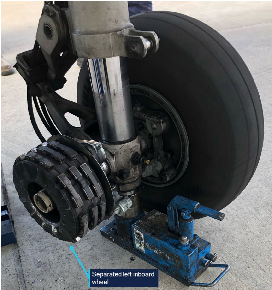
Figure 1: VH-VEZ left main landing gear with separated inboard wheel
