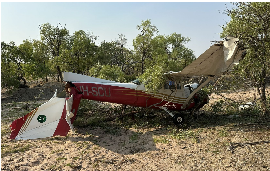
Figure 2: VH-SCU as it came to rest following impact with trees and terrain
