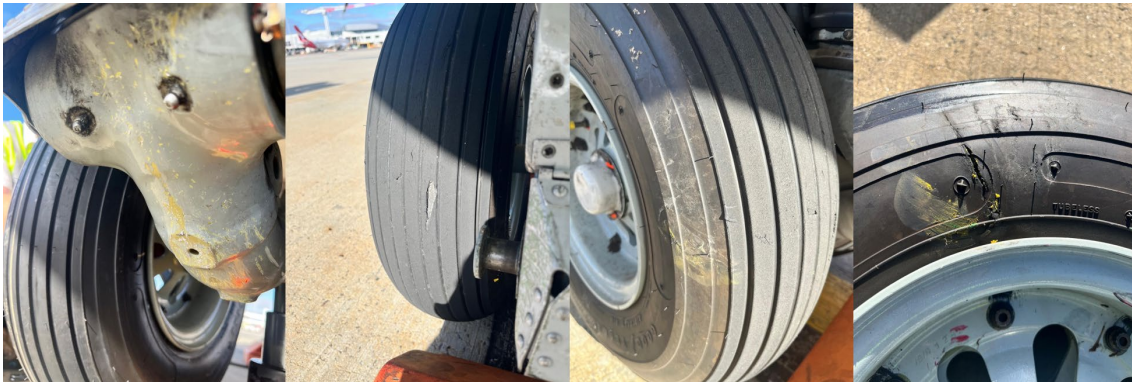
Figure 3: Nose landing gear damage
