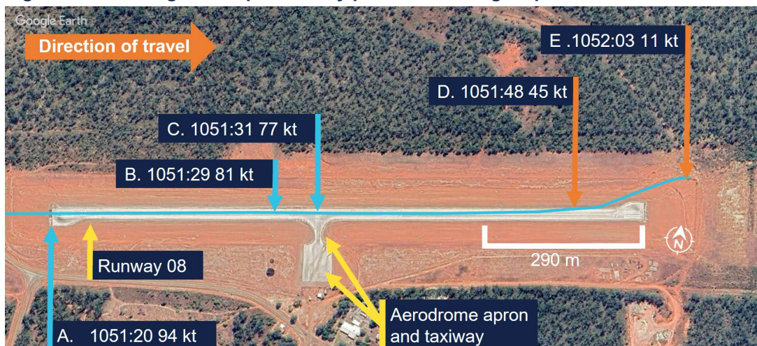
Figure 2: VH-NXA ground speed at key points in landing sequence
