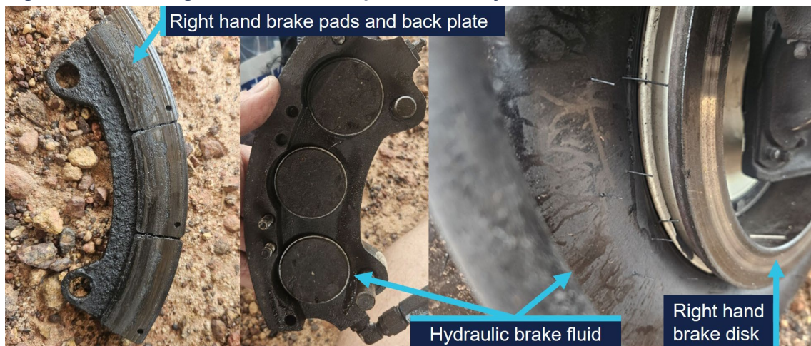
Figure 5: VH-NXA right hand brake components and hydraulic brake fluid
