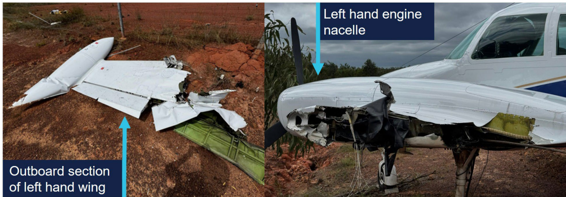
Figure 4: VH-NXA damaged left wing
