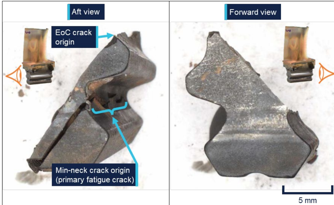
Figure 6: Dovetail of blade 50 recovered from the HPT disc
