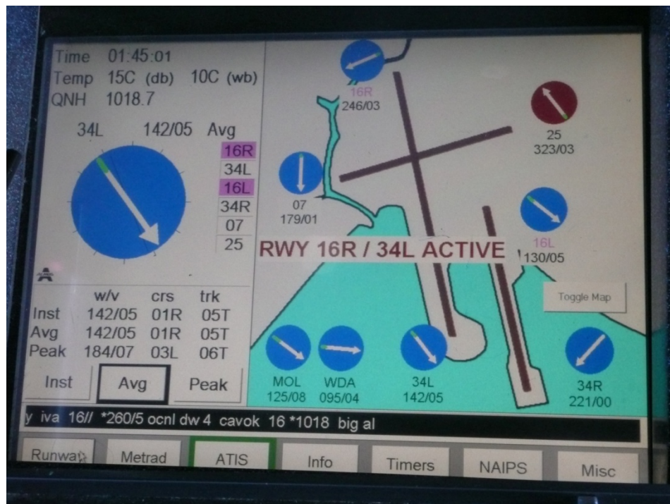
Figure 2: Sydney Control Tower surface wind display
