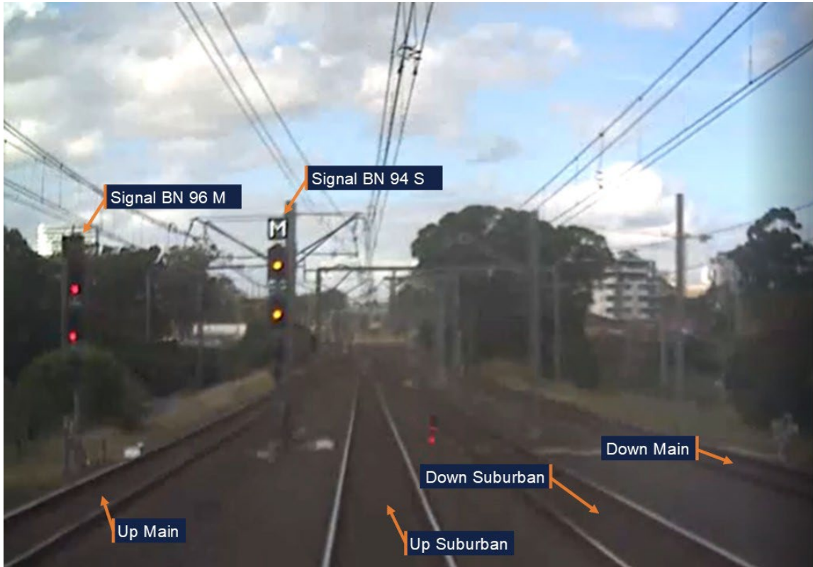
Image from Front of Train CCTV Car D6432 on incident run, approaching signal BN 94 S. Source: Sydney Trains, annotated by OTSI
