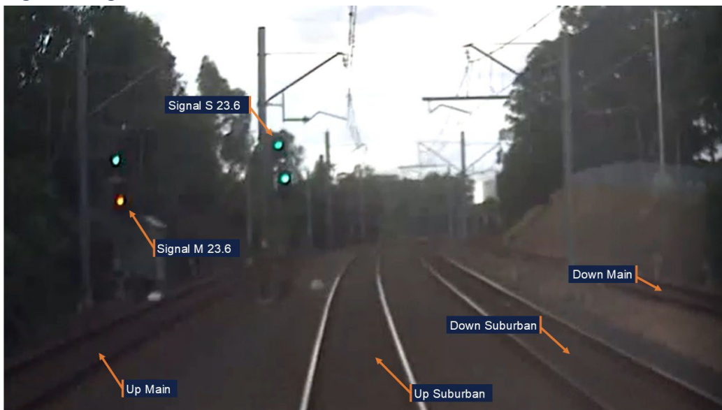
Image from Front of Train CCTV Car D6432 on incident run, approaching signal S 23.6. Source: Sydney Trains, annotated by OTSI
