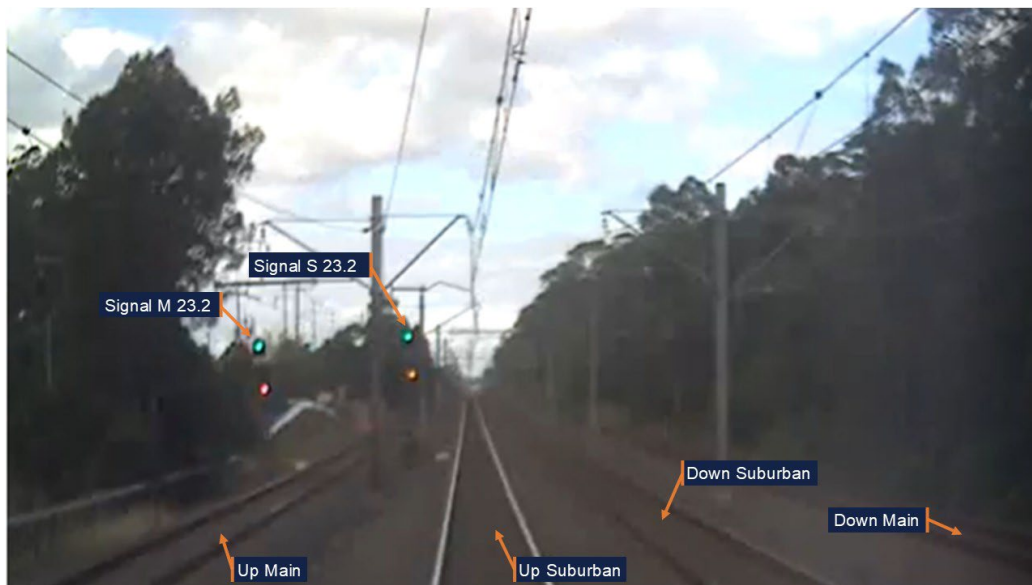
Image from Front of Train CCTV Car D6432 on incident run, approaching signal S 23.2. Source: Sydney Trains, annotated by OTSI
