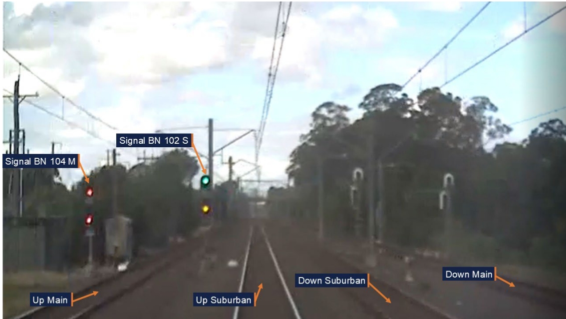
Image from Front of Train CCTV Car D6432 on incident run, approaching signal BN 102 S. Source: Sydney Trains, annotated by OTSI
