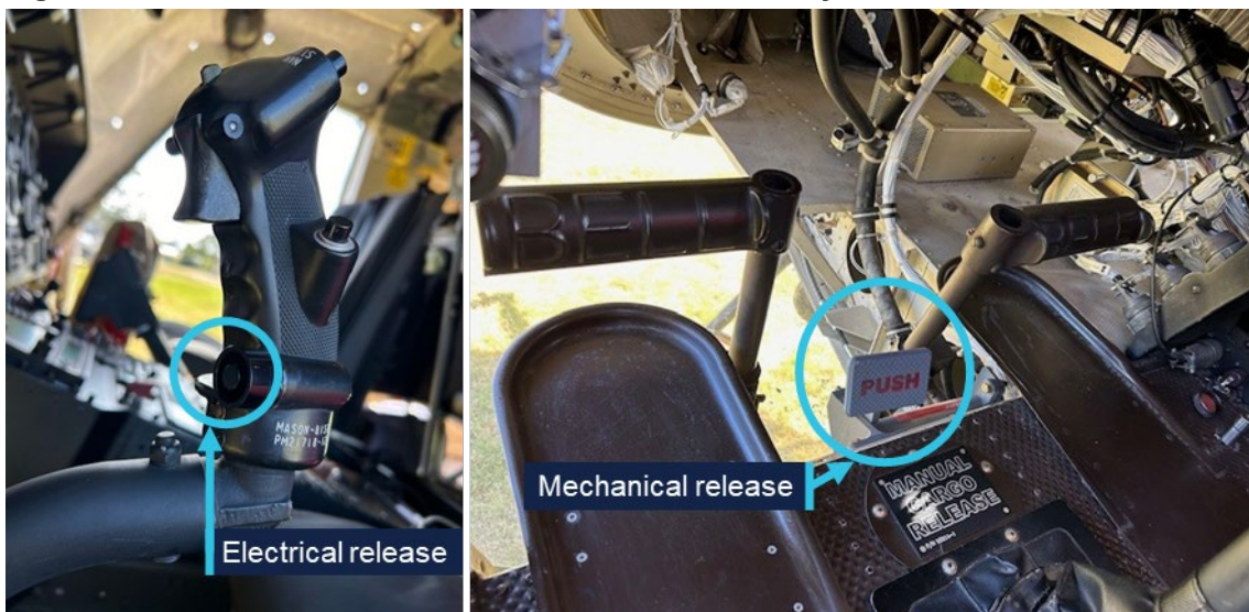
Figure 5: Electrical and mechanical external load release systems
