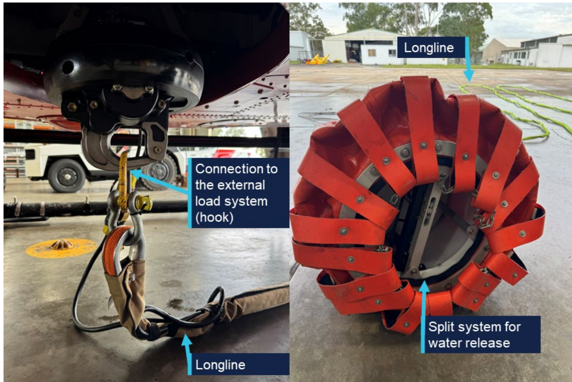
Figure 7: Longline attachment and Bambi Max bucket
