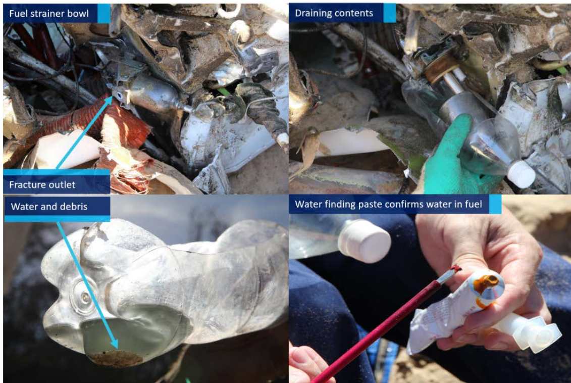
Figure 10: Fuel strainer bowl and contents showing signs of water and debris
