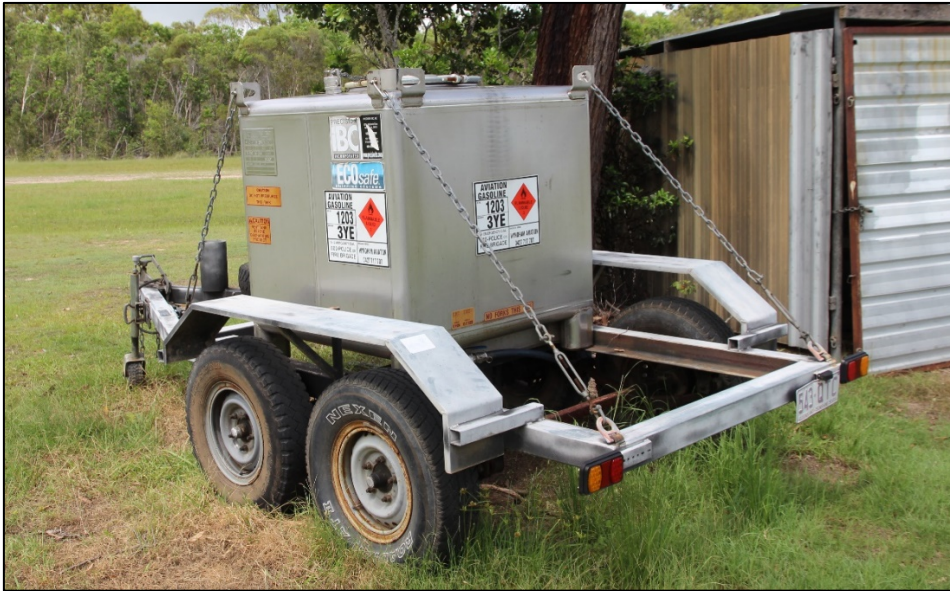
Figure 15: Fuel storage tank containing aviation grade gasoline
