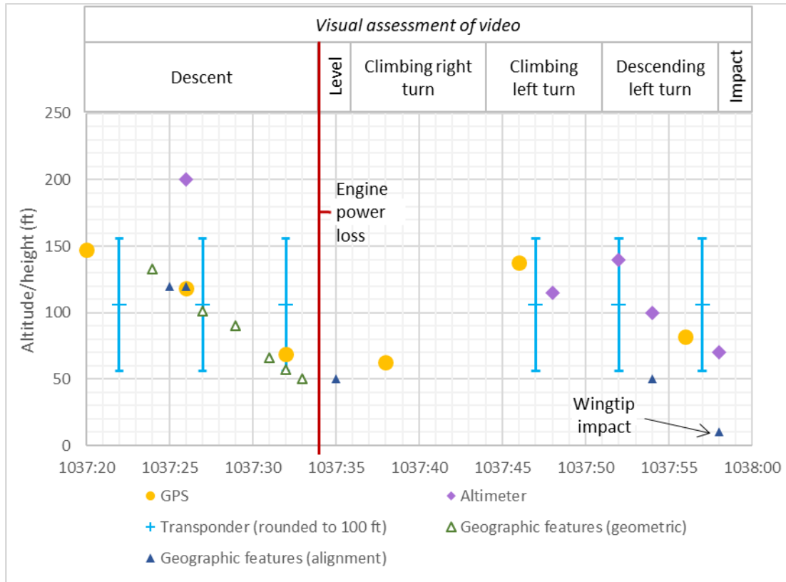
Figure B5: Summary of information about the aircraft’s altitude from 1037:20 until impact
