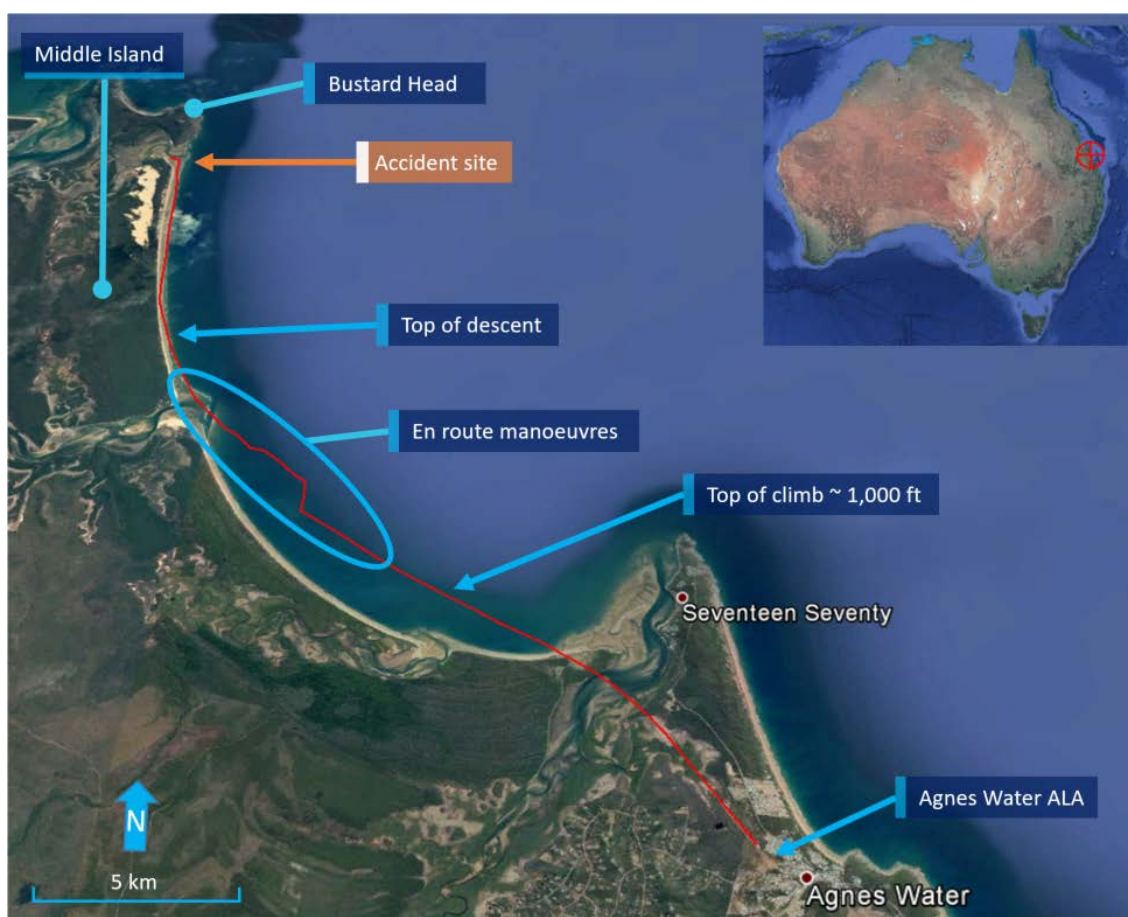
Figure 1: VH-WTQ's flight path between Agnes Water ALA and the accident location on Middle Island
