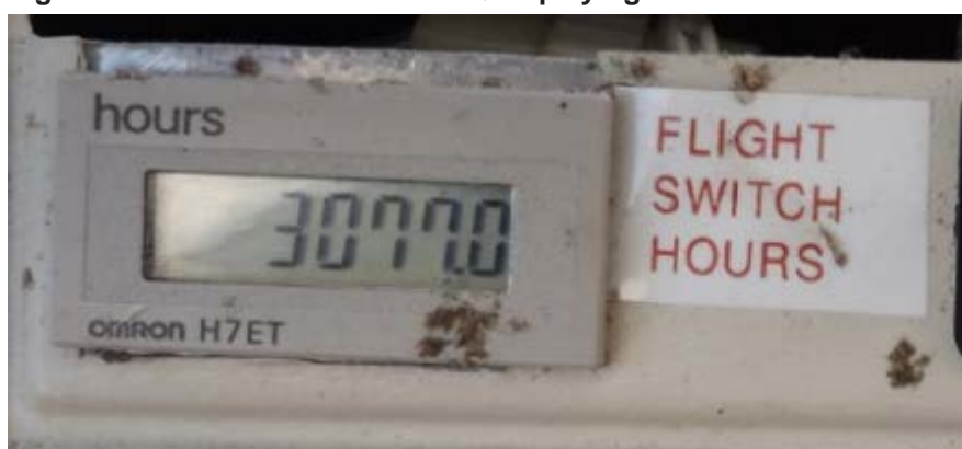
Figure A1: Hour meter on VH-WTQ displaying the value at the time of impact
