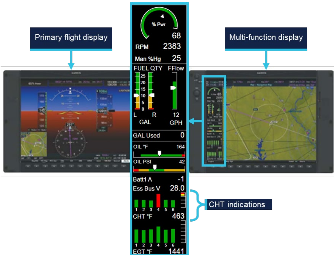
Figure 7: MFD engine indication system (EIS) panel, showing the vertical coloured bars indicating a CHT warning state for engine cylinder 4 temperature
