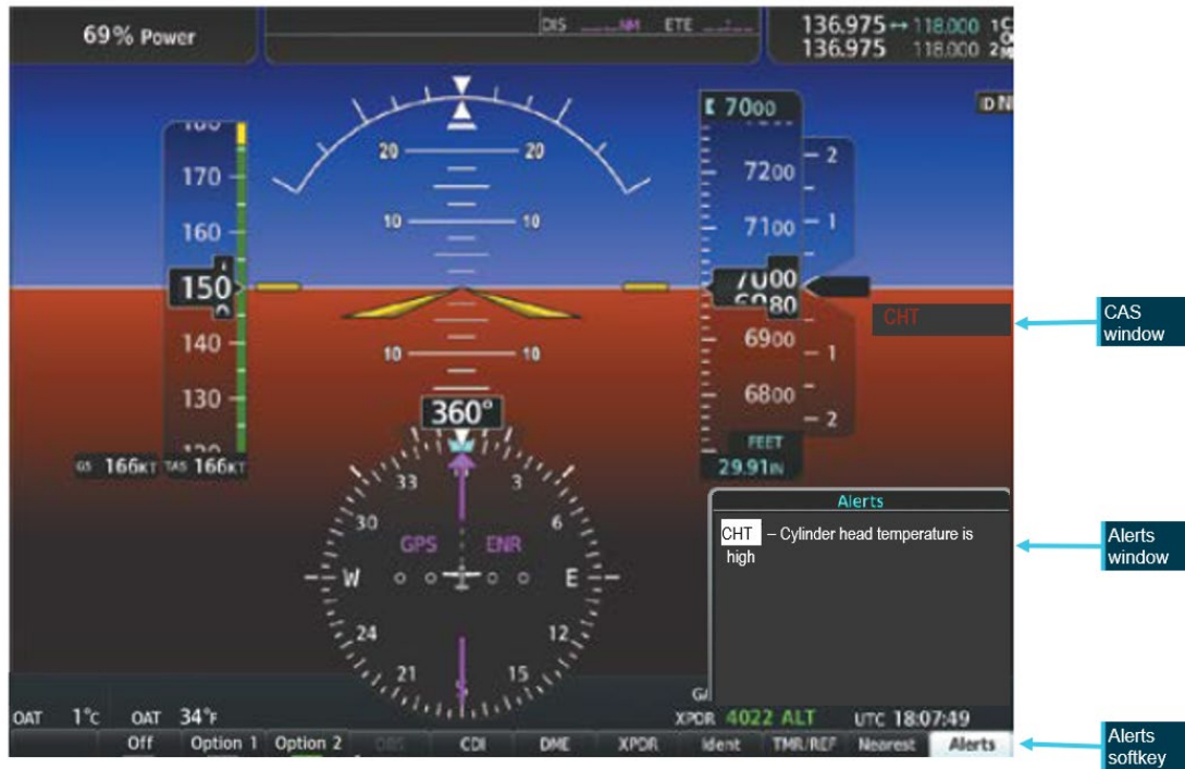
Figure 8: Exemplar window showing the crew alerting system (CAS) location and text for a CHT warning, the highlighted alerts softkey, and related alerts window text
