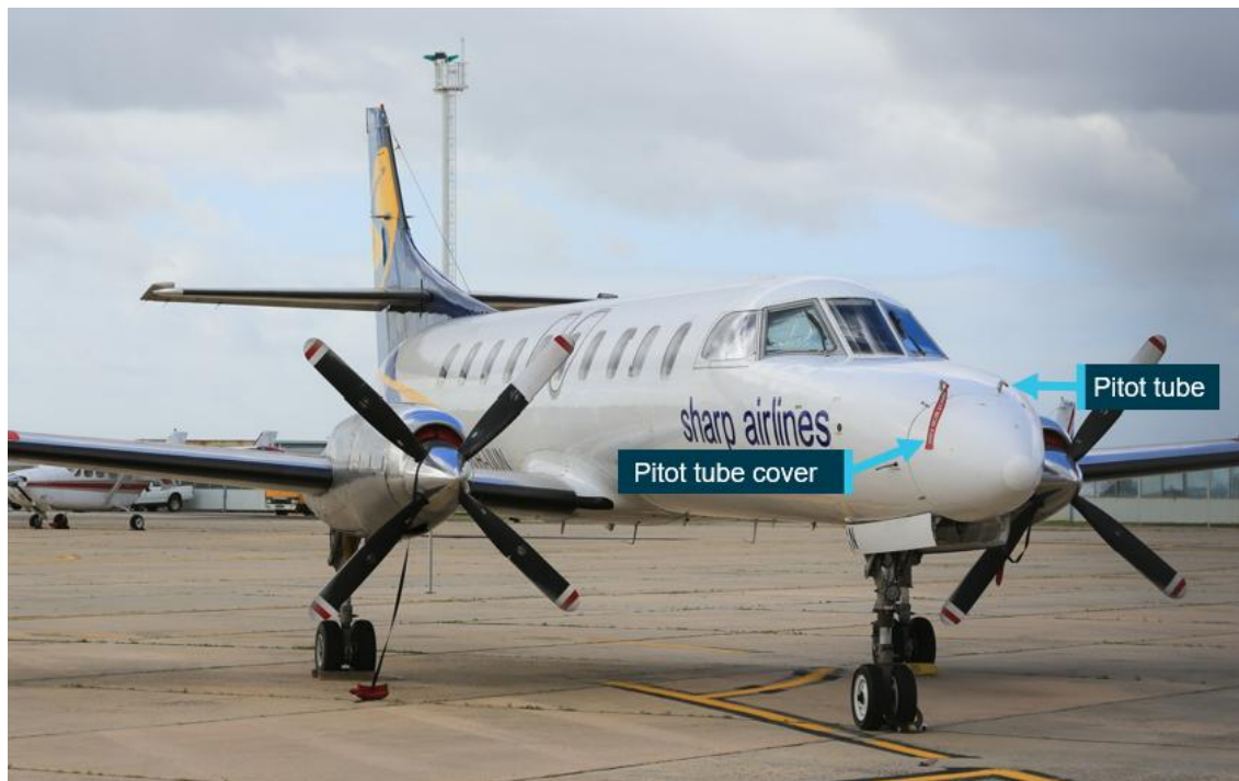
Figure 1: Pitot tubes on Fairchild SA227
