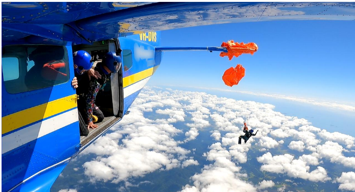
Figure 7: Reserve canopy torn and parachutist detached from aircraft
