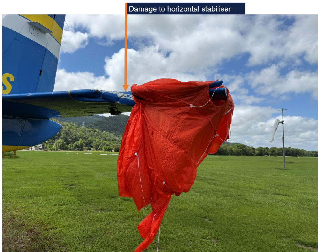
Figure 9: VH-DVS after landing, showing damage to the horizontal stabiliser
